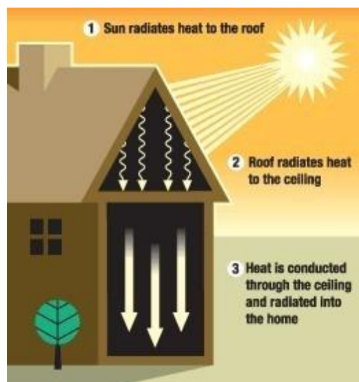
Figure 5.5: Illustration of radiation heat transfer
