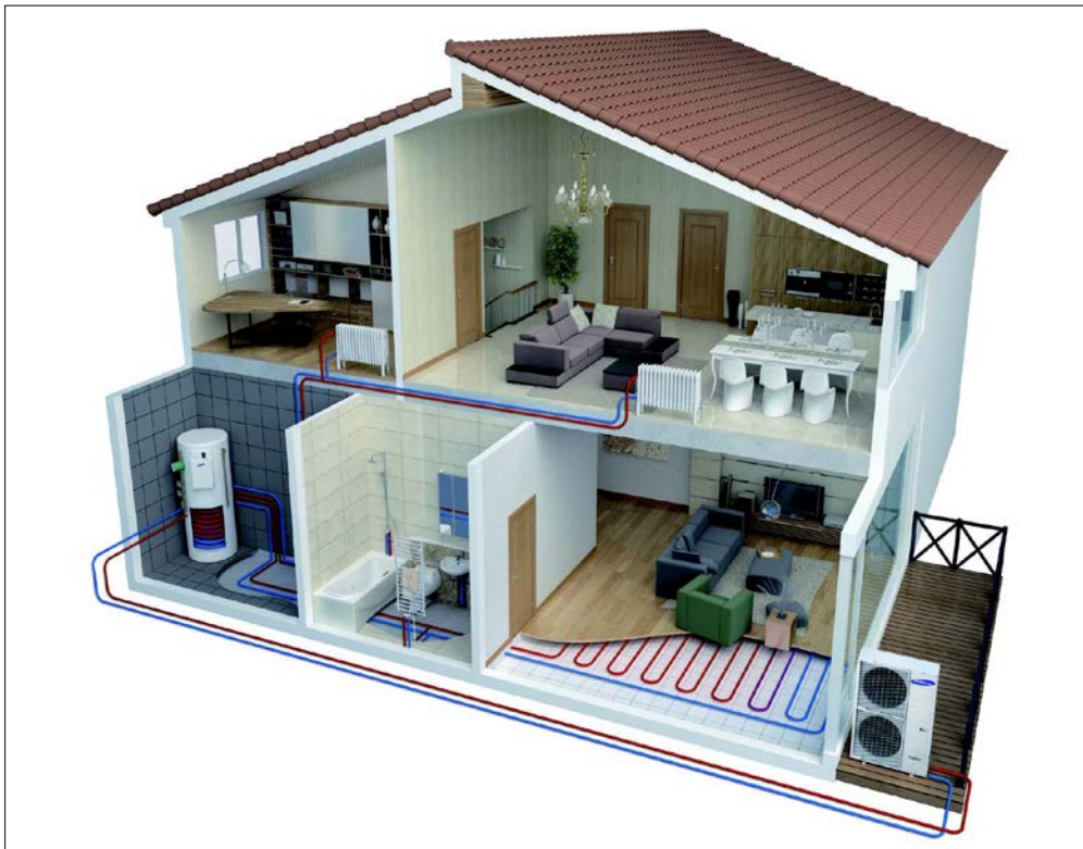
Figure e: Example of Air Source Heat Pump Installation 7
