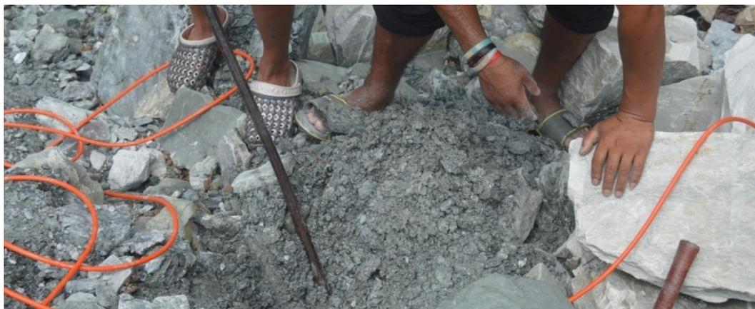
Field Photo 2 - Sampling of the soil and rock from the slide area
