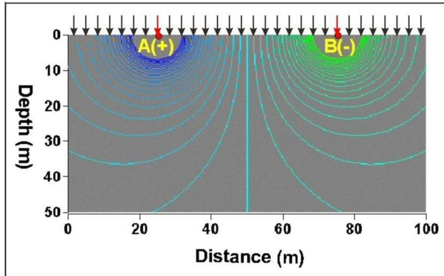
Figure 2. Schematic diagram showing the principle of the resistivity method.
