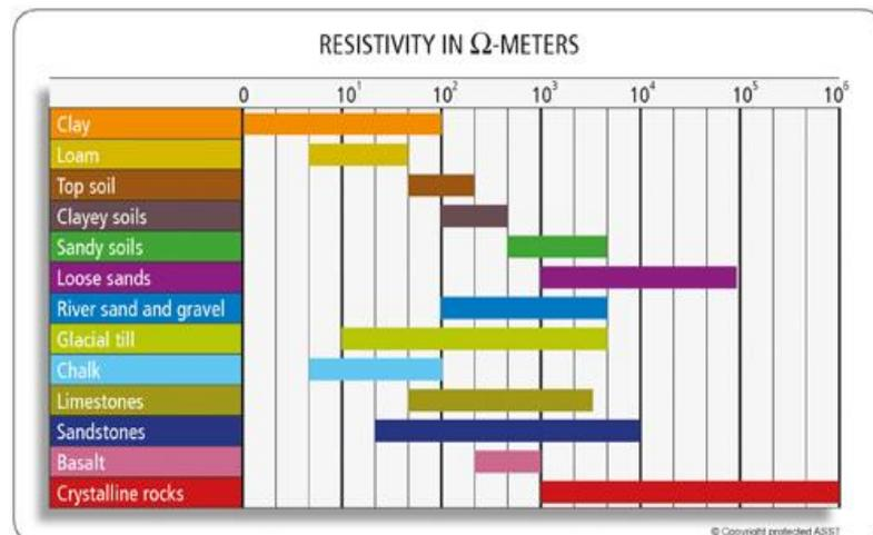
Figure 15. Typical values of resistivity of materials (Applied Scientific Service and Technology).
