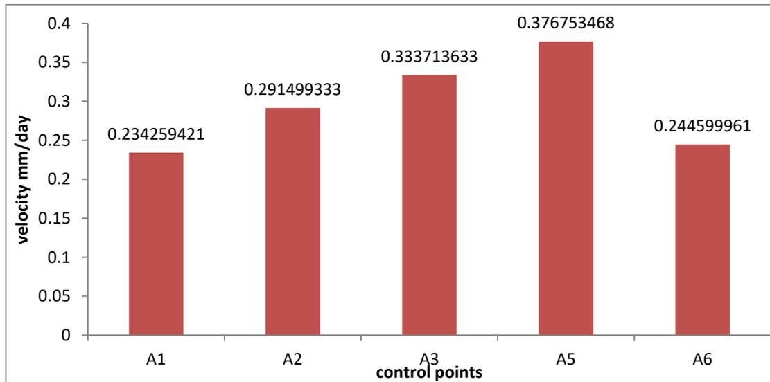
Figure 7. Graph showing the rate of movement of control points at Arong landslide
