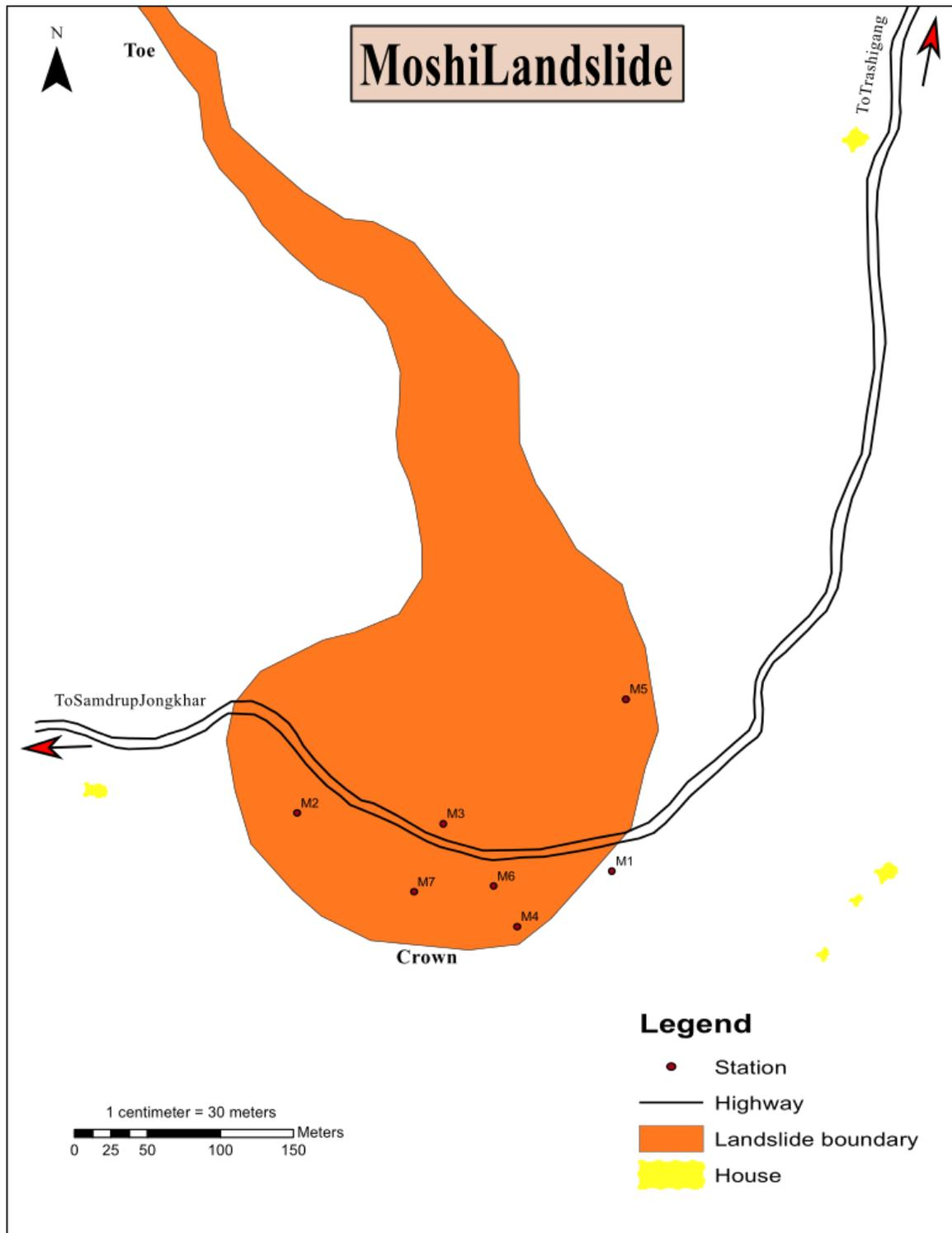
Figure 3. Moshi landslide map showing prominent feature along with the locations of GPS observation points
