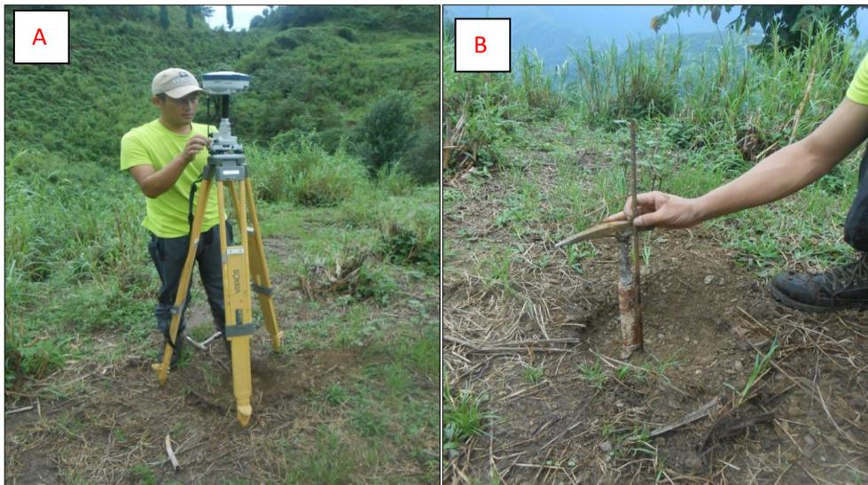
Figure 6. A) GPS used for the observation of points at Arong. B) 60 cm rod used to mark the GPS station points with a geological hammer for scale.
