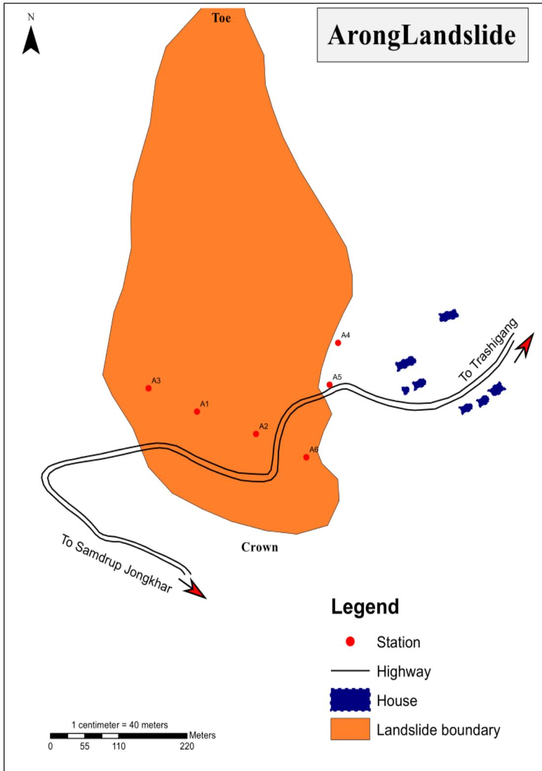
Figure 2. Arong landslide map showing prominent features and location of GPS observation points.
