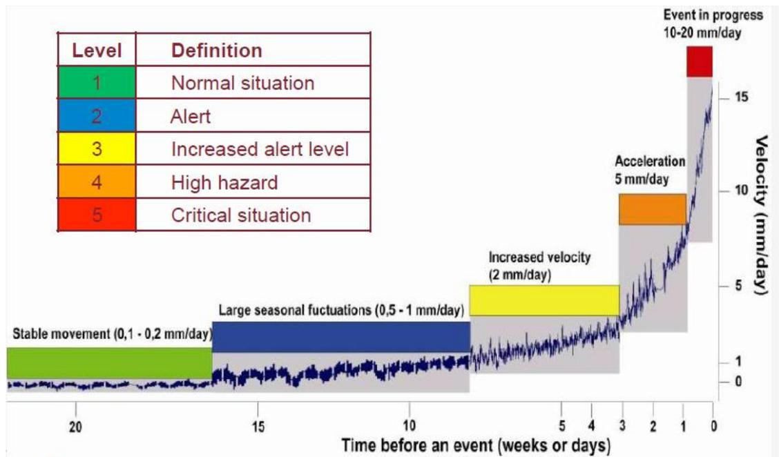
Figure 14. The relationship between landslide movement rate and situational or hazard levels.
