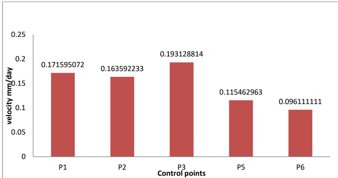
Figure 9. Graph showing the rate of movement of control points at the Phongmey landslide.
