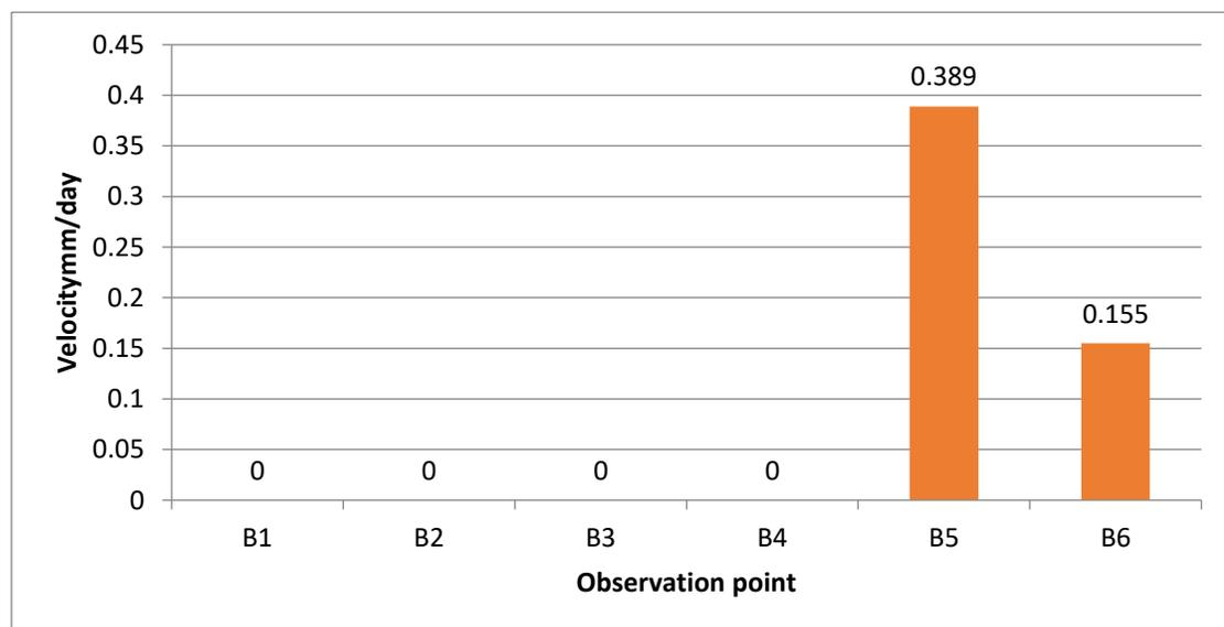
Figure 8. Graph showing the rate of movement of control points at Box-cutting landslide
