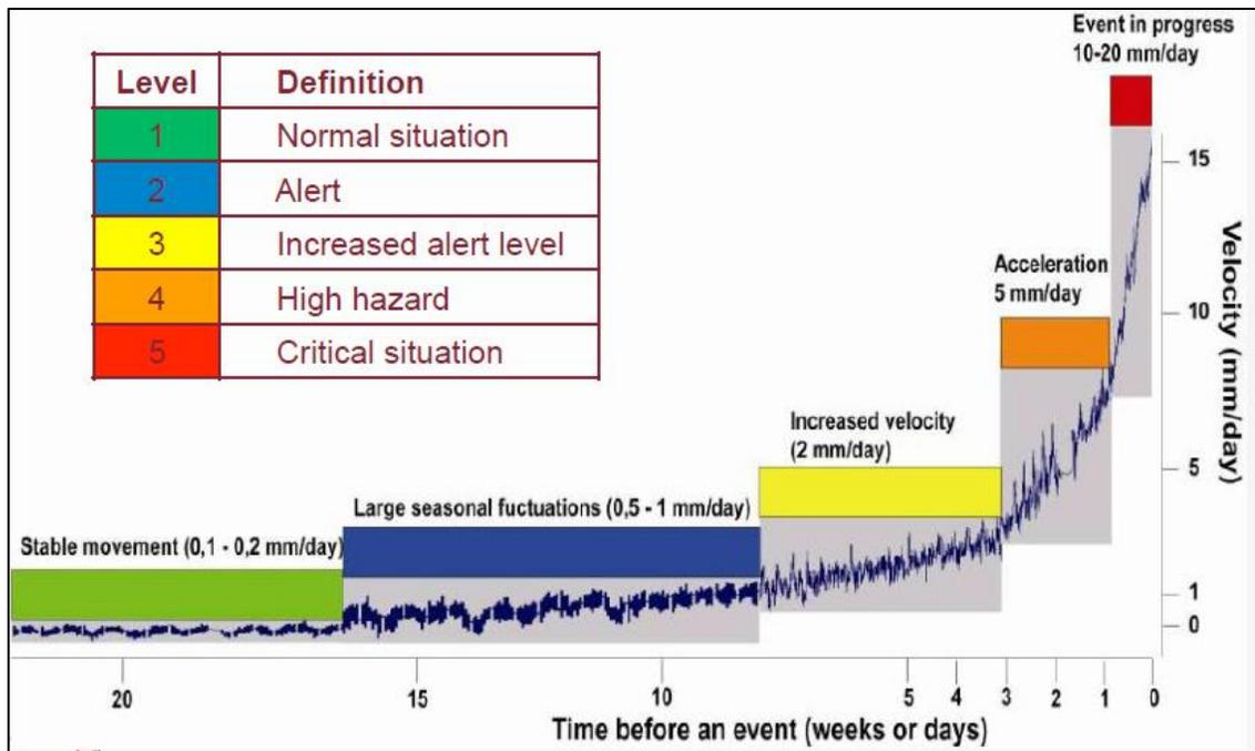
Figure 14. The relationship between landslide movement rate and situational or hazard levels
