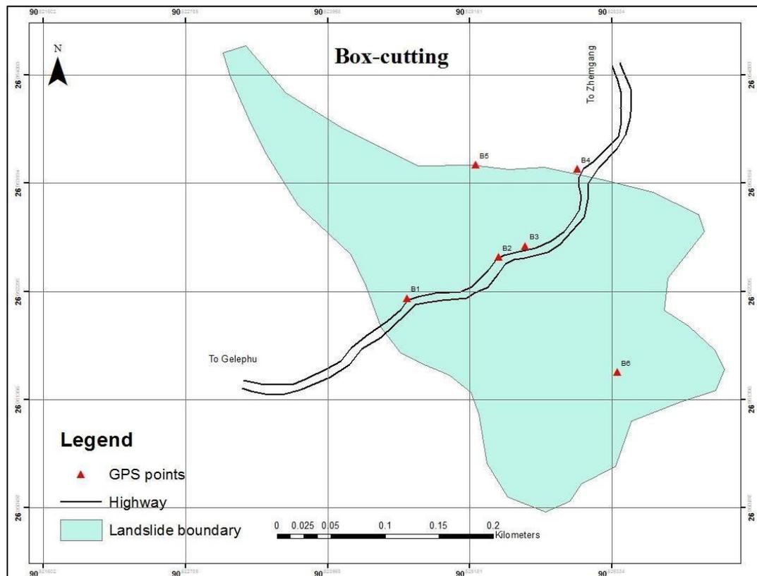
Figure 4. Box-cutting landslide map showing prominent features and location of GPS Observation points.
