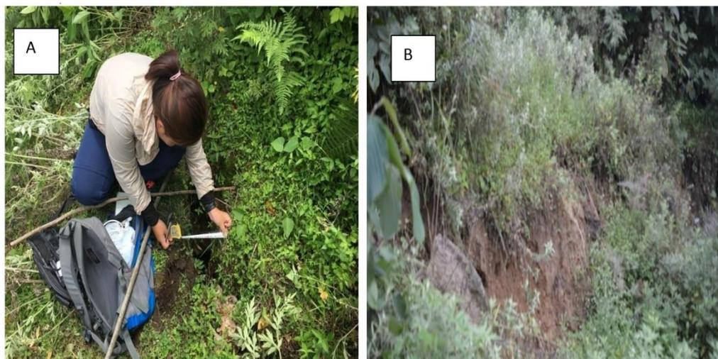
*Figure 9. Tension crack developed on the crown of the landslide at Tsimasham (Picture taken in May 2016) and (B) showing displaced crack (Picture taken in May 2017).*
