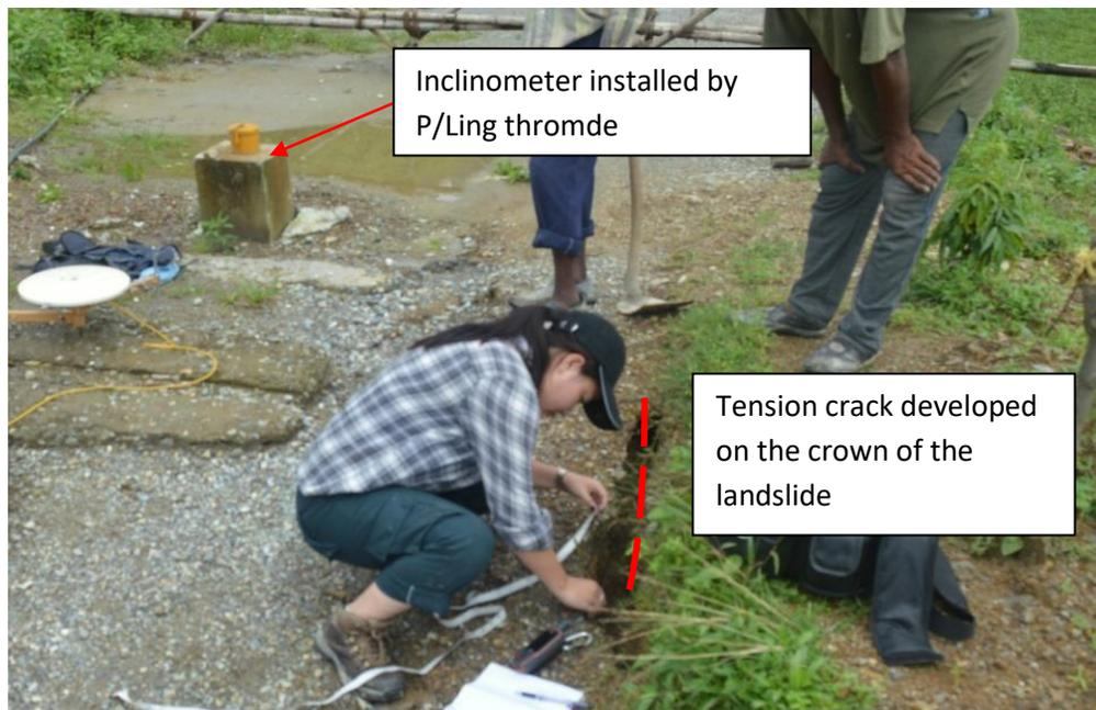
Figure 11. Tension crack developed at Reldri shown by red dotted line (Picture taken in August 2015)
