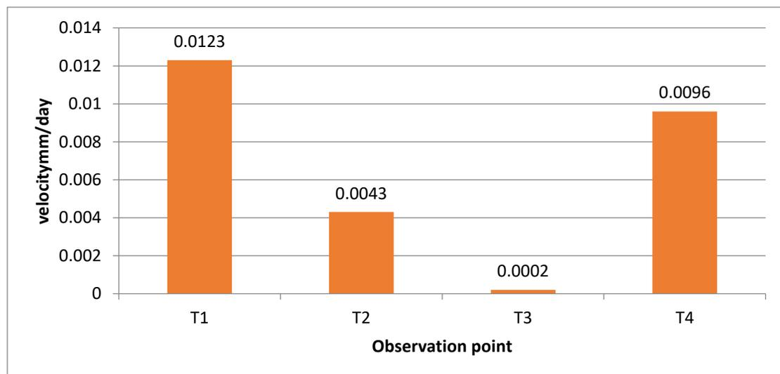
Figure 6. Graph showing the rate of movement of control points at Tsimasham landslide.
