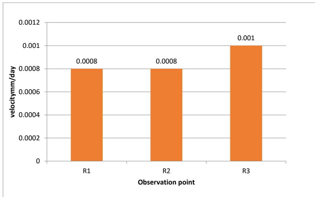
Figure 7. Graph showing the rate of movement of control points at Reldri landslide
