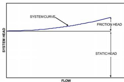
*Figure 44: System curve with high static head*
