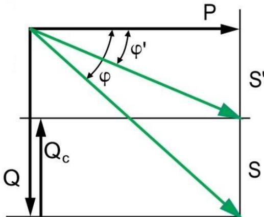
Figure 11: Power factor correction triangle
