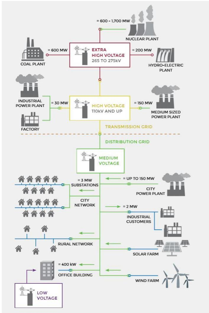
Figure 5: Illustration of electricity transmission and distribution system (Source: UNEP)
