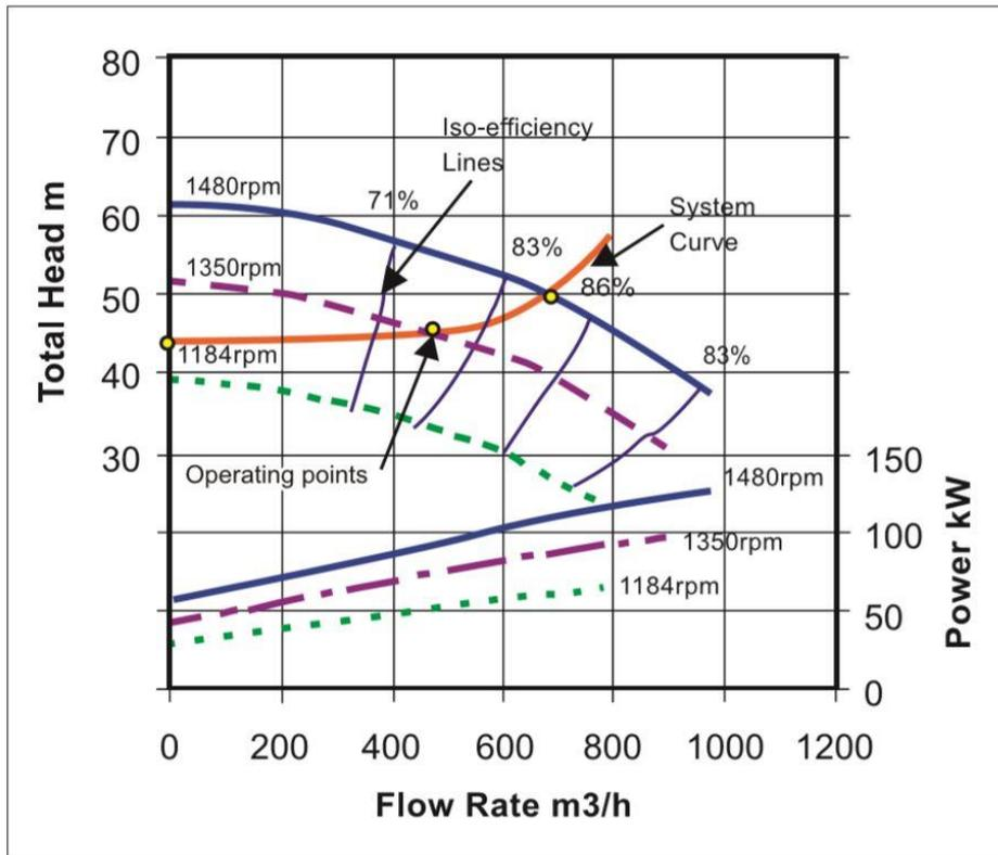
Figure 52: Effect of speed change in a system with high static head
