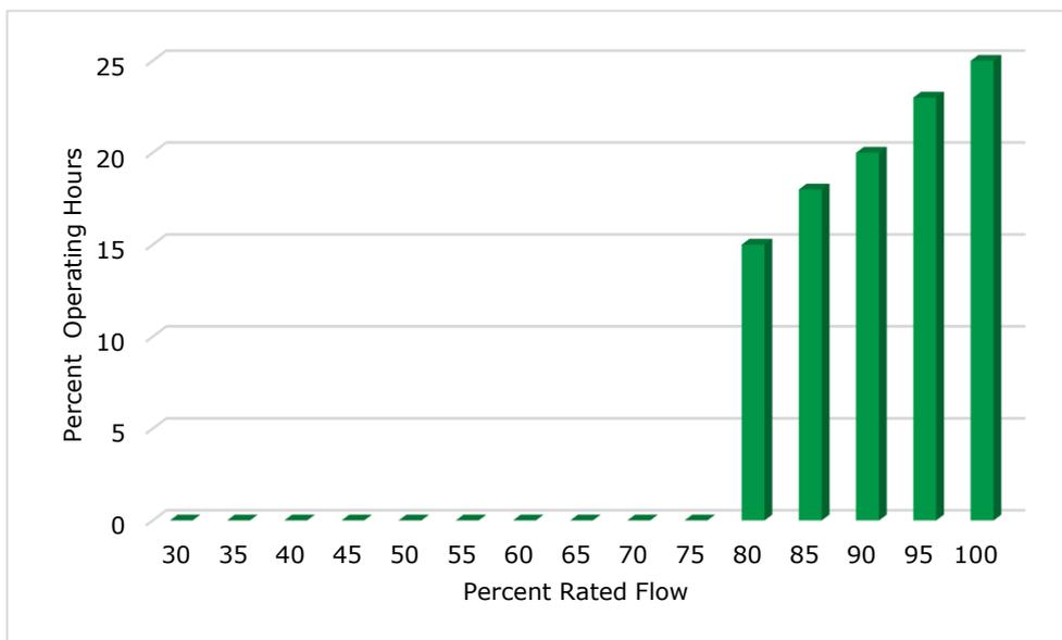
Figure 25: Example of a poor variable speed drive candidate
