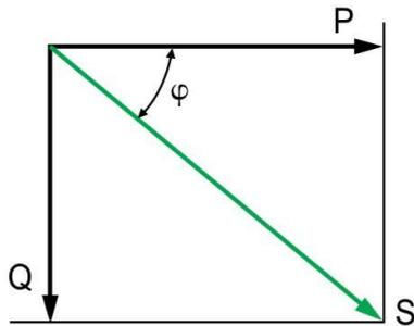
$$\cos \phi = \frac{P \text{ (kW)}}{S \text{ (kVA)}}$$
