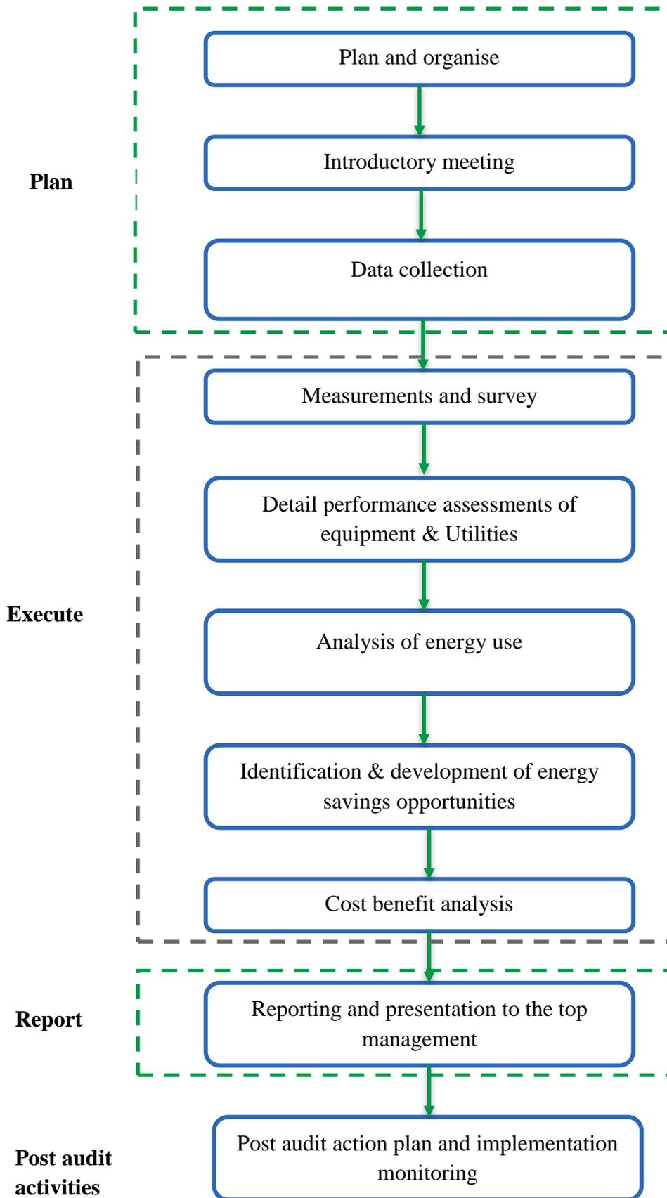
Figure 1: Overview of detail energy audit procedure
