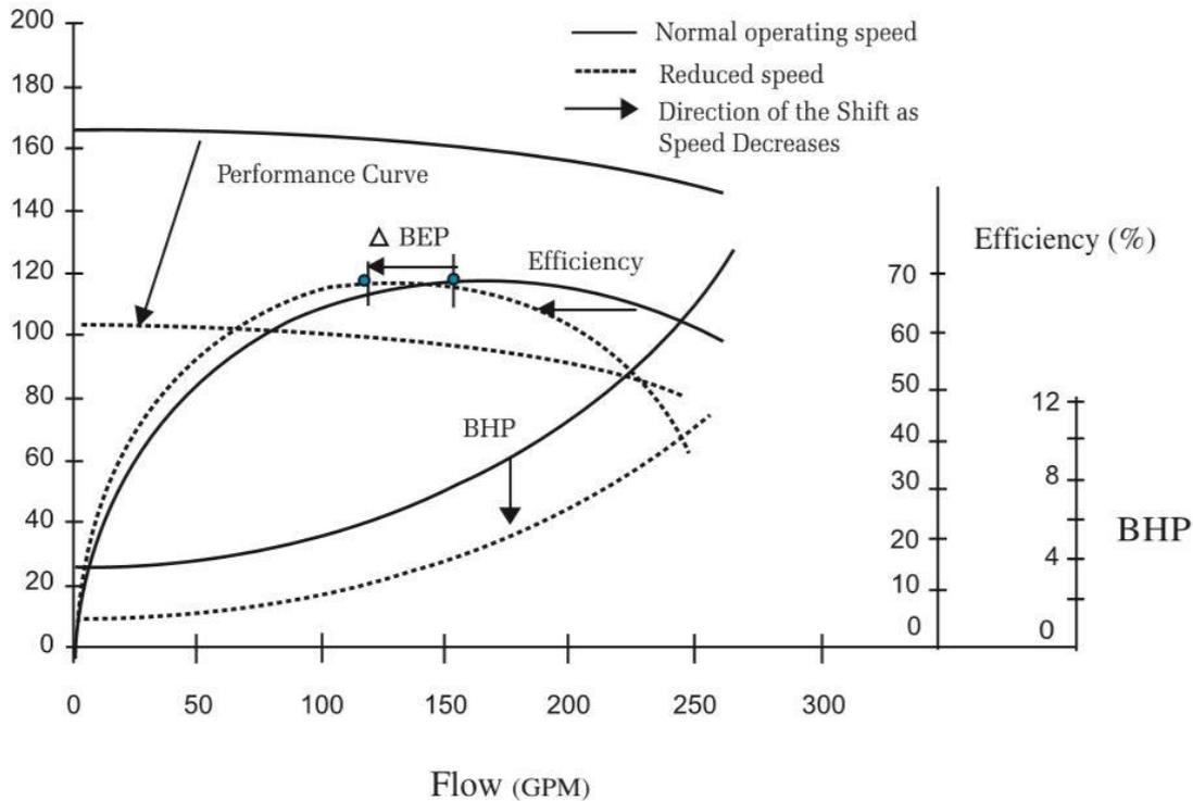
Figure 53: Effect of VFD
