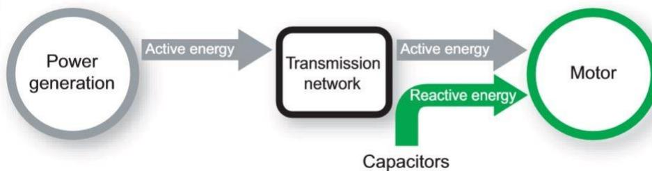
Figure 9: Connection of capacitors at load level
