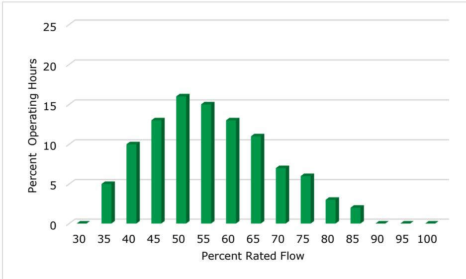
Figure 24: Example of an excellent variable speed drive candidate
