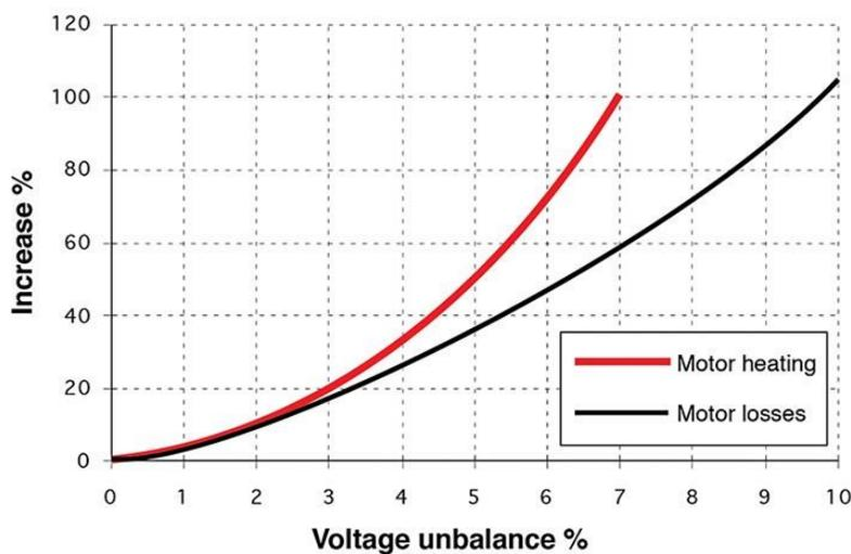
Figure 14: Voltage unbalance (%) versus motor losses & motor heating (Source: BEE)
