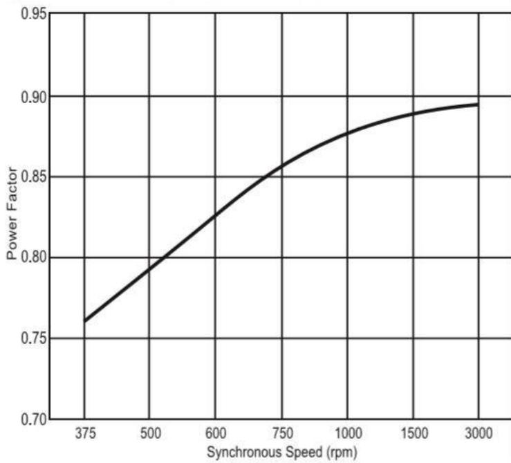
Figure 16: Effect of motor speed on power factor (Source: BEE)
