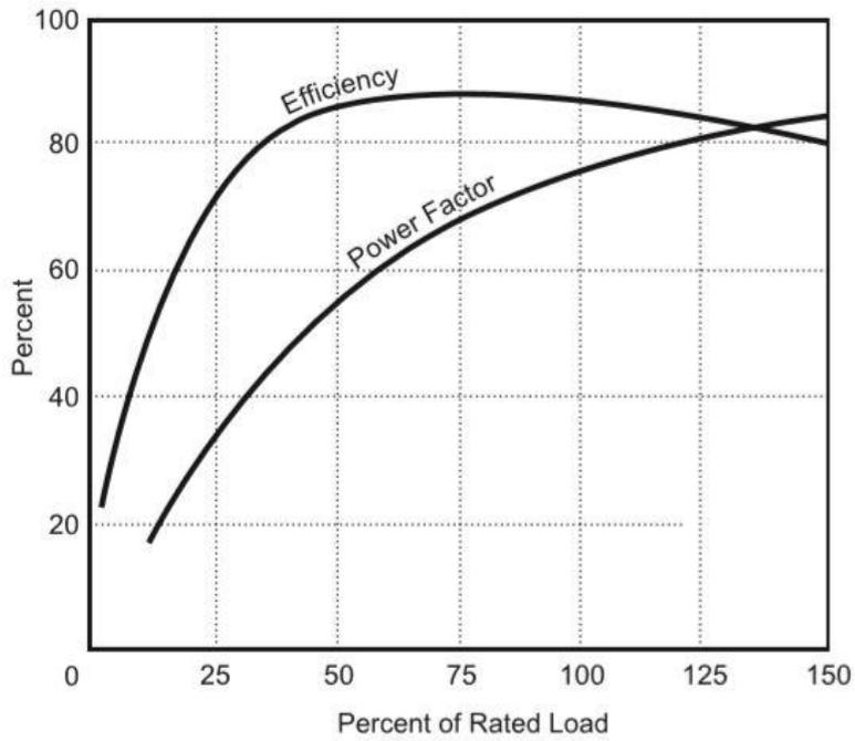
Figure 15: Effect of motor loading on efficiency & power factor (Source: BEE)
