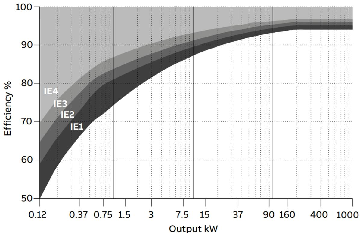
Figure 22: IE efficiency classes for 4 pole motors at 50 Hz (Source: ABB)
