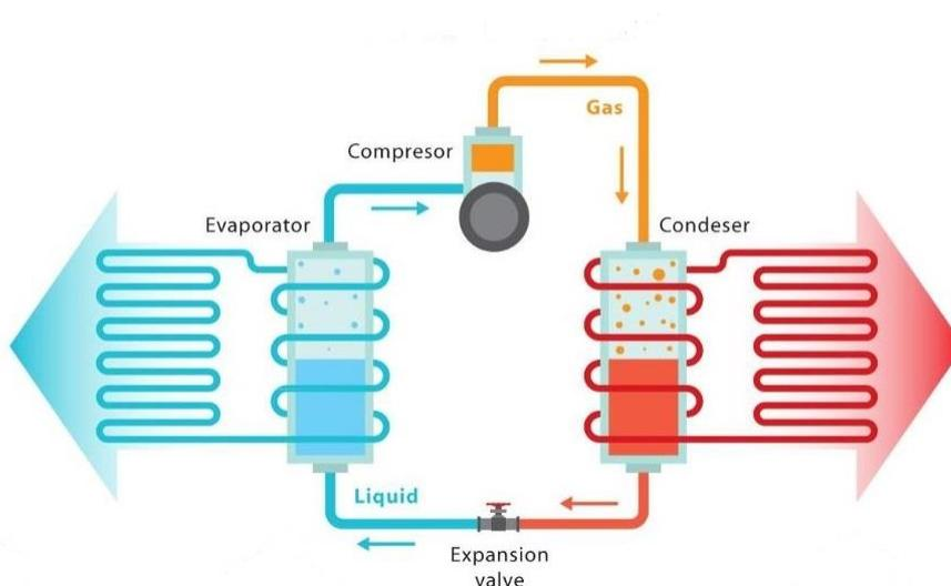
Figure 28: Vapour compression refrigeration system
