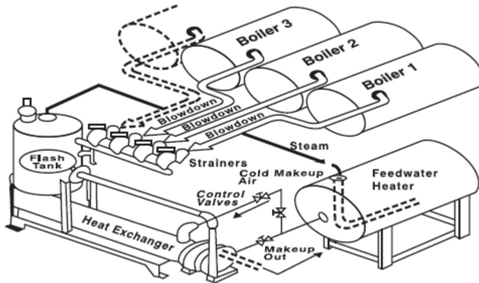
Figure 59: Blowdown heat recovery system
