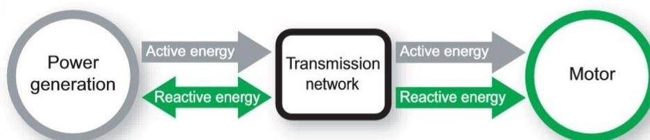
*Figure 7: Reactive energy supplied and billed by the energy supplier or utility*
