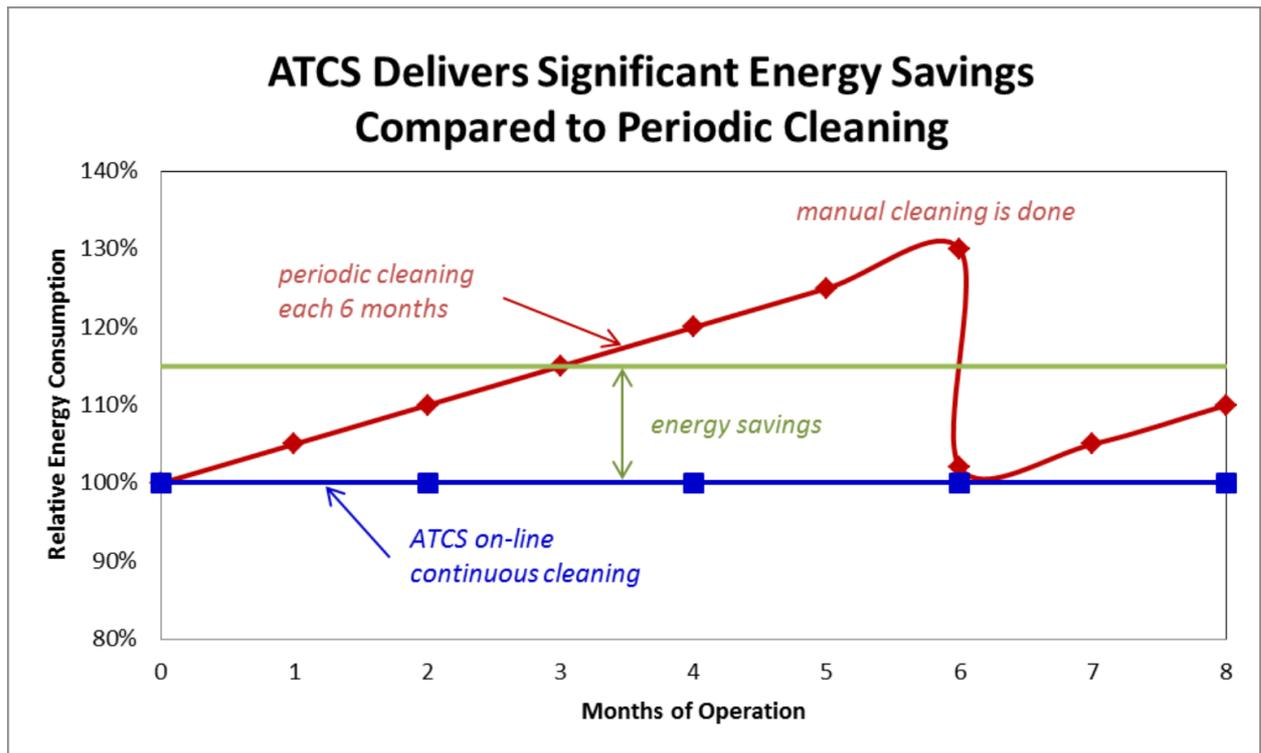
Figure 30: Benefit of automatic tube cleaning system (Source: Trane)
