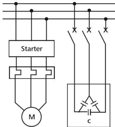
*Figure 21: Method 2 - Capacitor is connected to the motor before starter*
