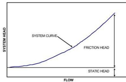
*Figure 45: System head with low static head*
