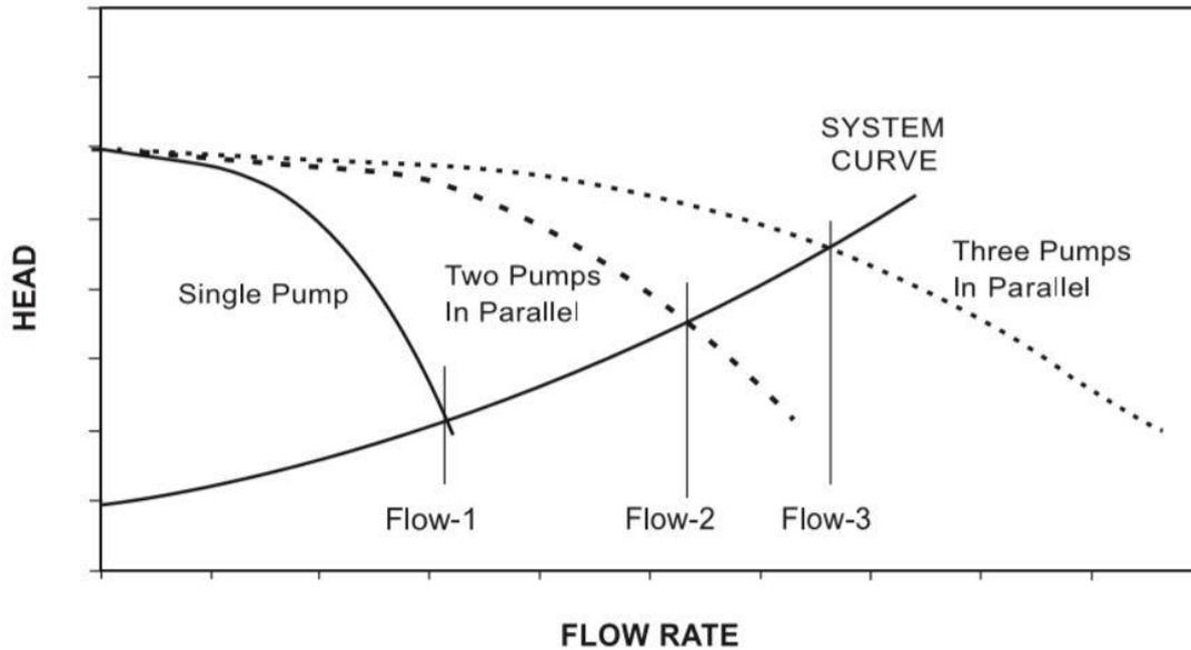
Figure 54: Typical head-flow curve for pumps in parallel operation
