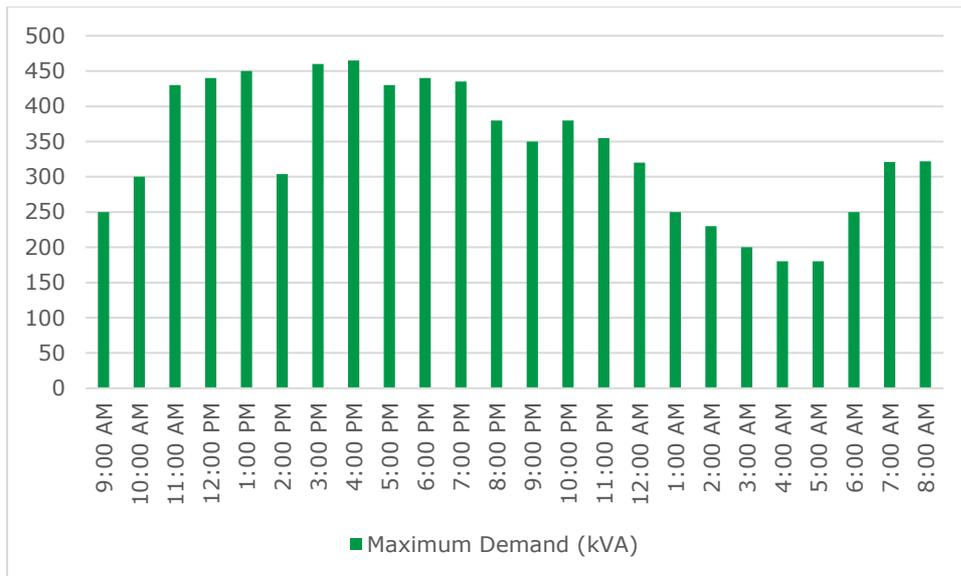
Figure 6: Hourly load curve
