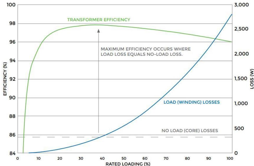
Figure 13: Transformer losses as a percentage (%) of load (Source: UNEP)
