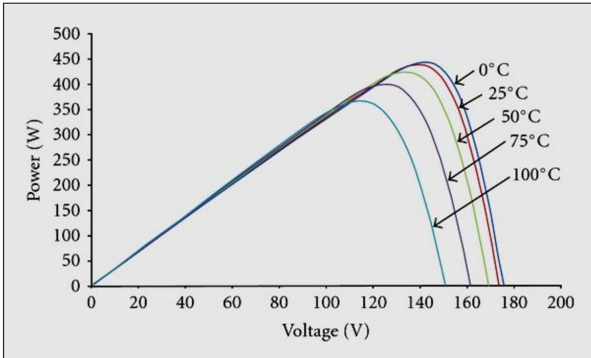
Figure 65: Effect of temperature change on power and voltage
