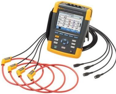
A three-phase power analyser with a yellow and black body, a large color display, and several red and black test leads. |
