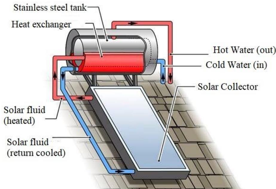
Figure 66: Solar water heater
