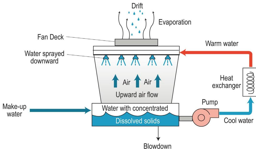
Figure 55: Cooling tower with closed loop
