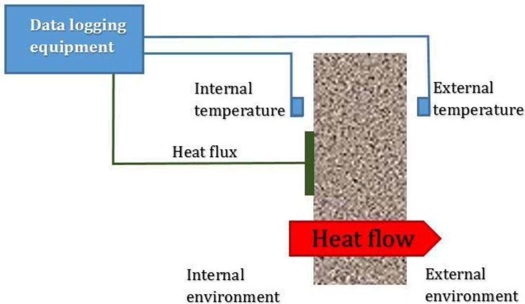
**Condition 1** — the duration of the test exceeds 72 hours (three days) if the temperature is stable around the
