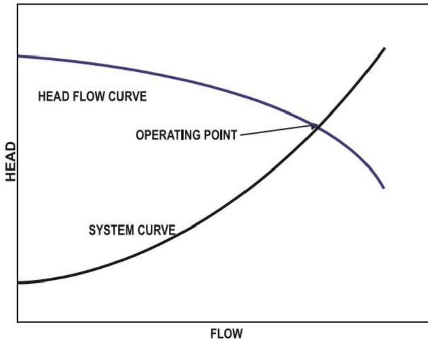
Figure 48: Pump operating point
