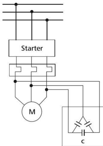
*Figure 20: Method 1- Capacitor is connected directly to the motor*
