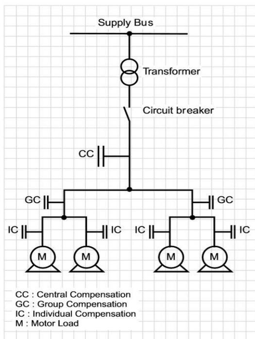
Figure 12: Different compensation modes for power factor improvement
