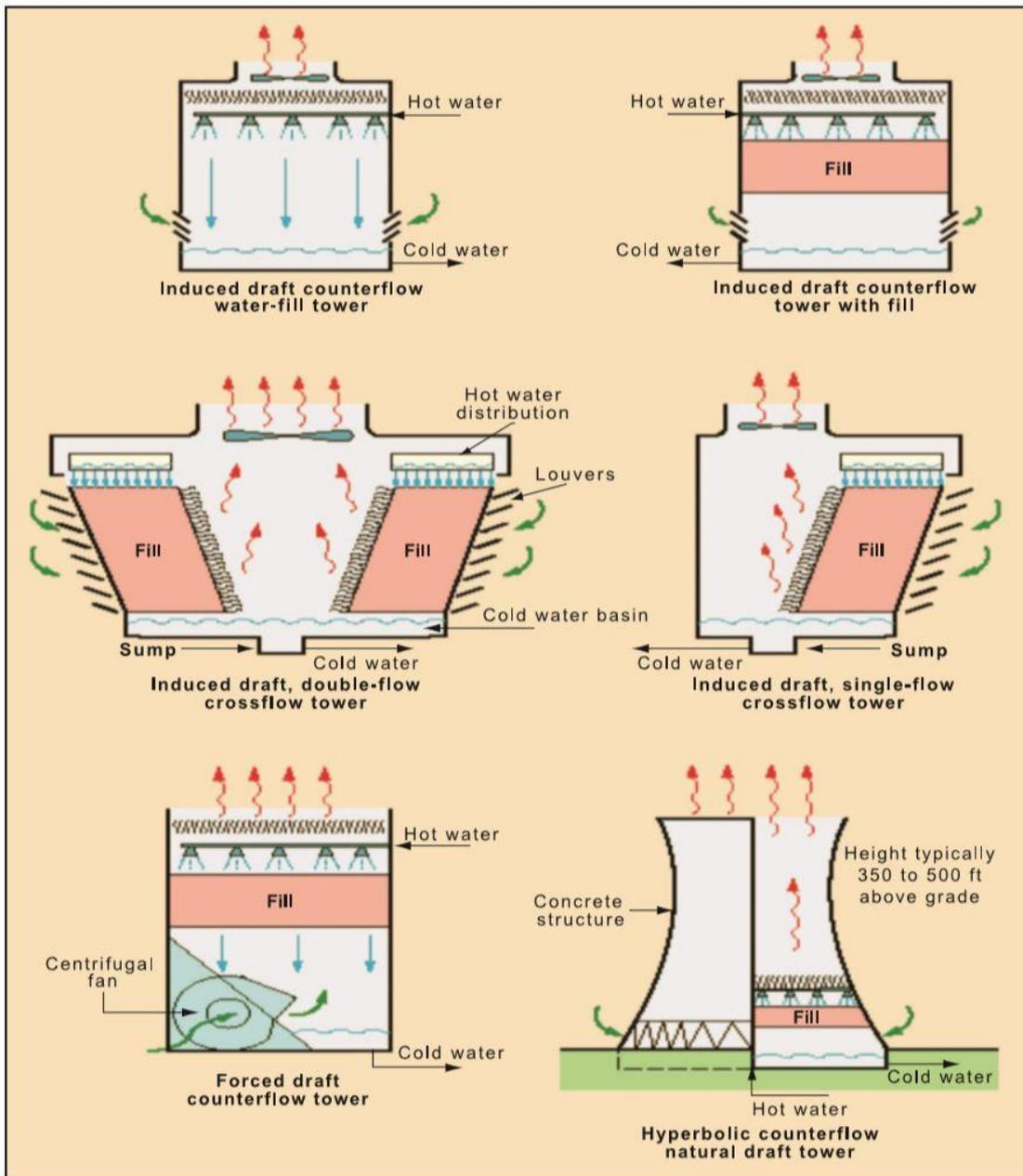
Figure 56: Types of cooling tower (Source: BEE)
