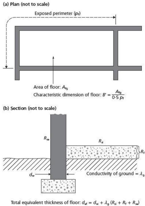
Figure 35: Total equivalent thickness of floor
