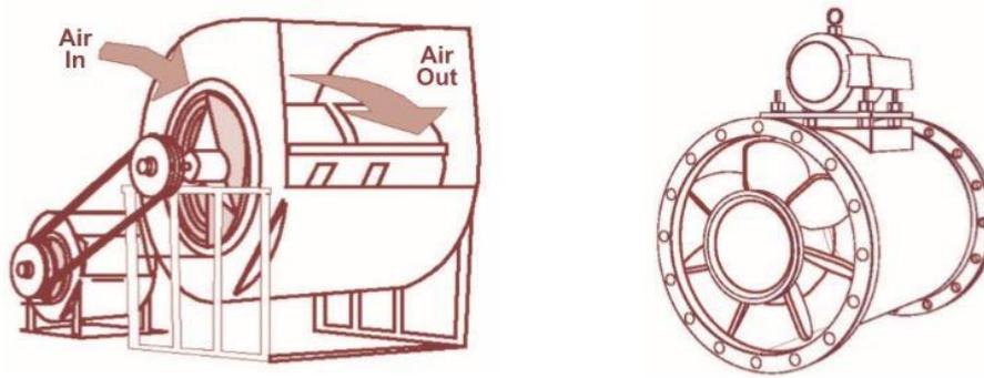
Figure 37: Centrifugal fan (left) and axial fan (right)
