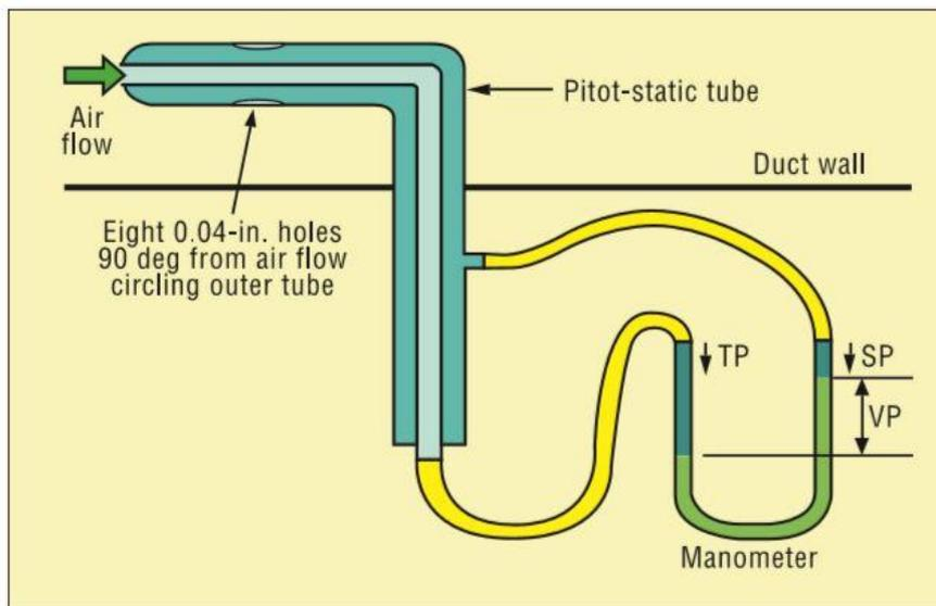
*Figure 38: Measurement by pitot tube*
