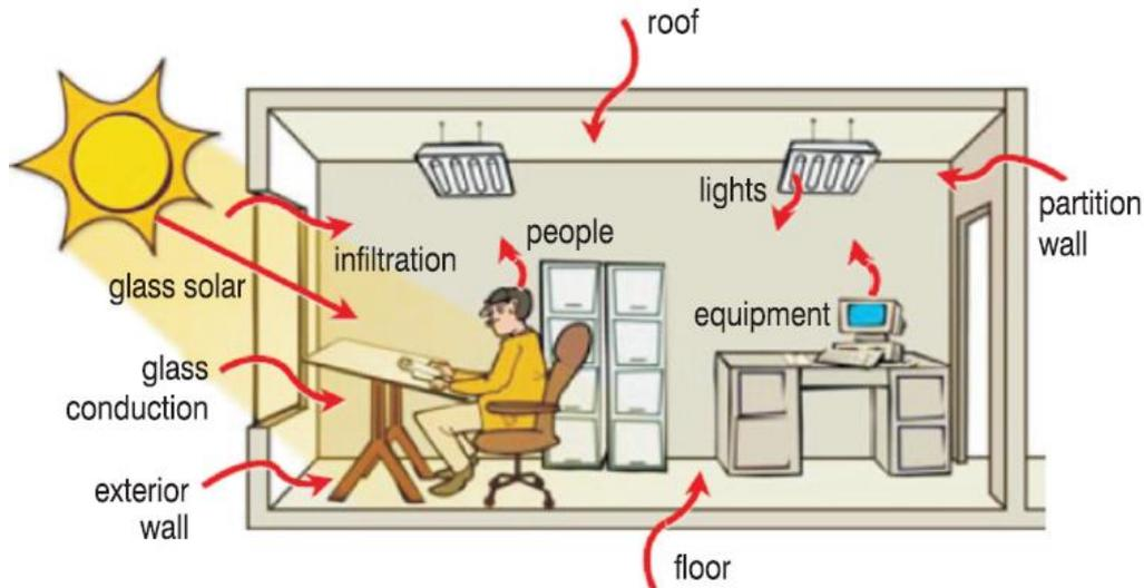
Figure 29: Heat gain sources in building envelope (Source: BEE)
