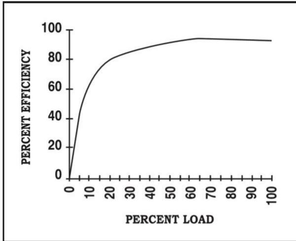
Figure 17: Effect of motor loading on efficiency (Source: BEE)
