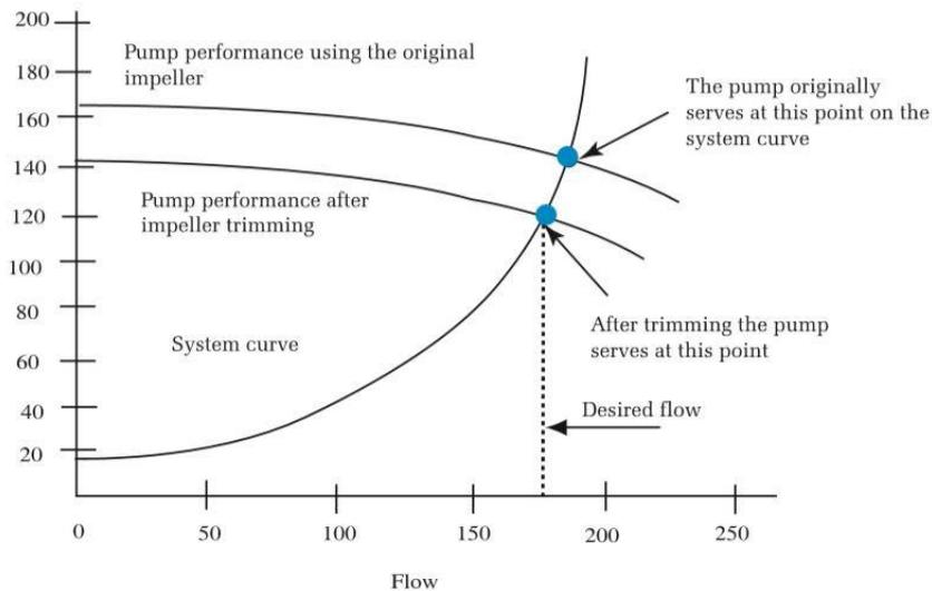
Figure 50: After impeller trimming
