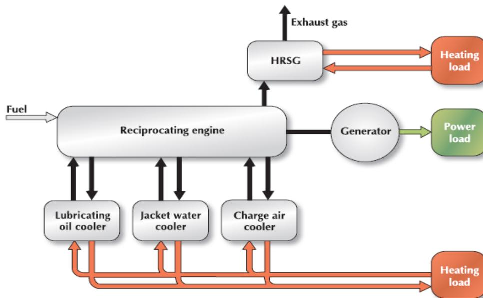
Figure 60: Reciprocating engine cogeneration
