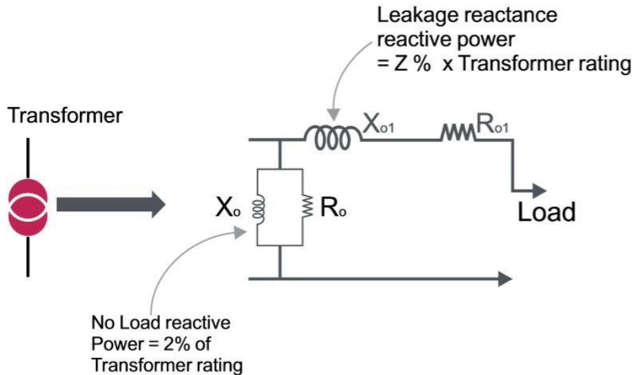
Figure 10: No-load compensation for transformer
