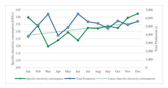
Figure 6: An example of line graph depicting specific electricity consumption (SEC) over time and increasing trend of SEC
