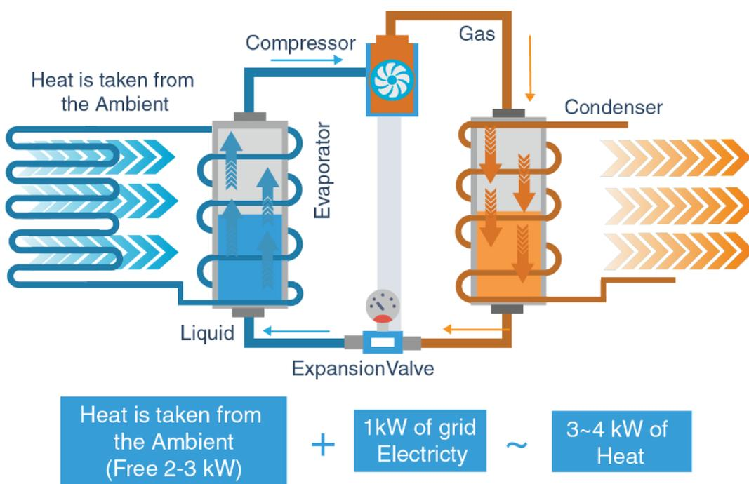
Figure 40: Heat Pump working (Source: Aspiration energy)
