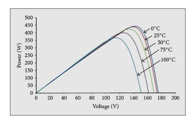
Figure 95: Effect of temperature change on power and voltage
