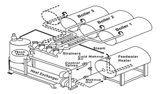
Figure 66: Blowdown heat recovery system
