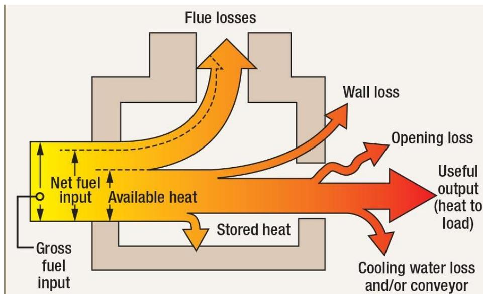
*Figure 70: Furnace losses*
