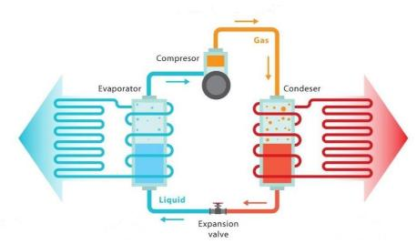
Figure 37: Vapour compression refrigeration system
