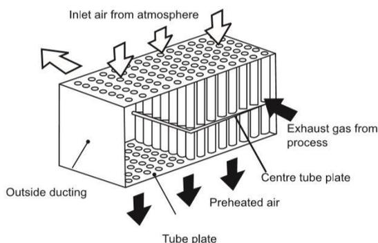
Figure 83: Recuperator configuration
