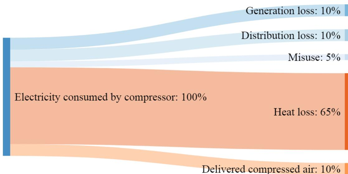
Figure 31: Sankey diagram of compressed air losses
