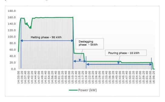
Figure 67: Different phases of induction furnace batch process – an example (Source: STENUM Asia)
