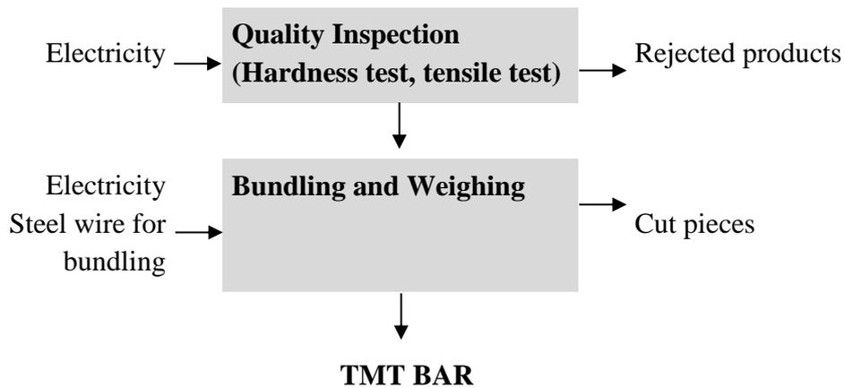
*Figure 2: An example of process flow chart*
