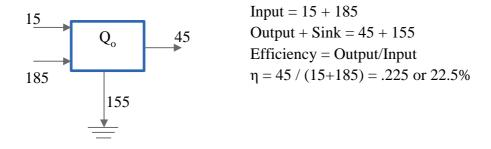
Figure 100: Efficiency and losses
