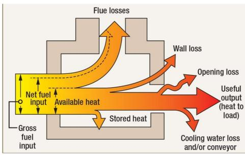
Figure 70: Furnace losses
