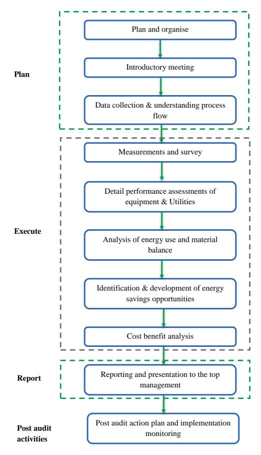
Figure 1: Overview of detail energy audit procedure
