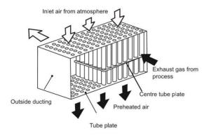
Figure 83: Recuperator configuration
