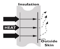
Figure 71: Furnace wall losses
