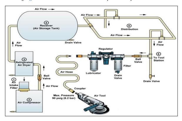
Figure 33: Figure of elements of compressed air system showing generation, distribution, and usage (Source: Gison Pneumatics)
