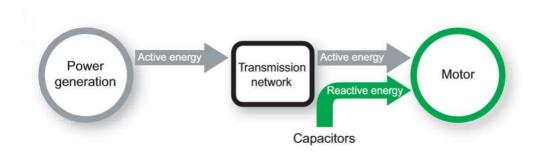
Figure 14: Connection of capacitors at load level
