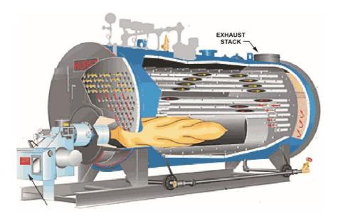
Figure 64: Packaged Boiler (Source: BEE)
