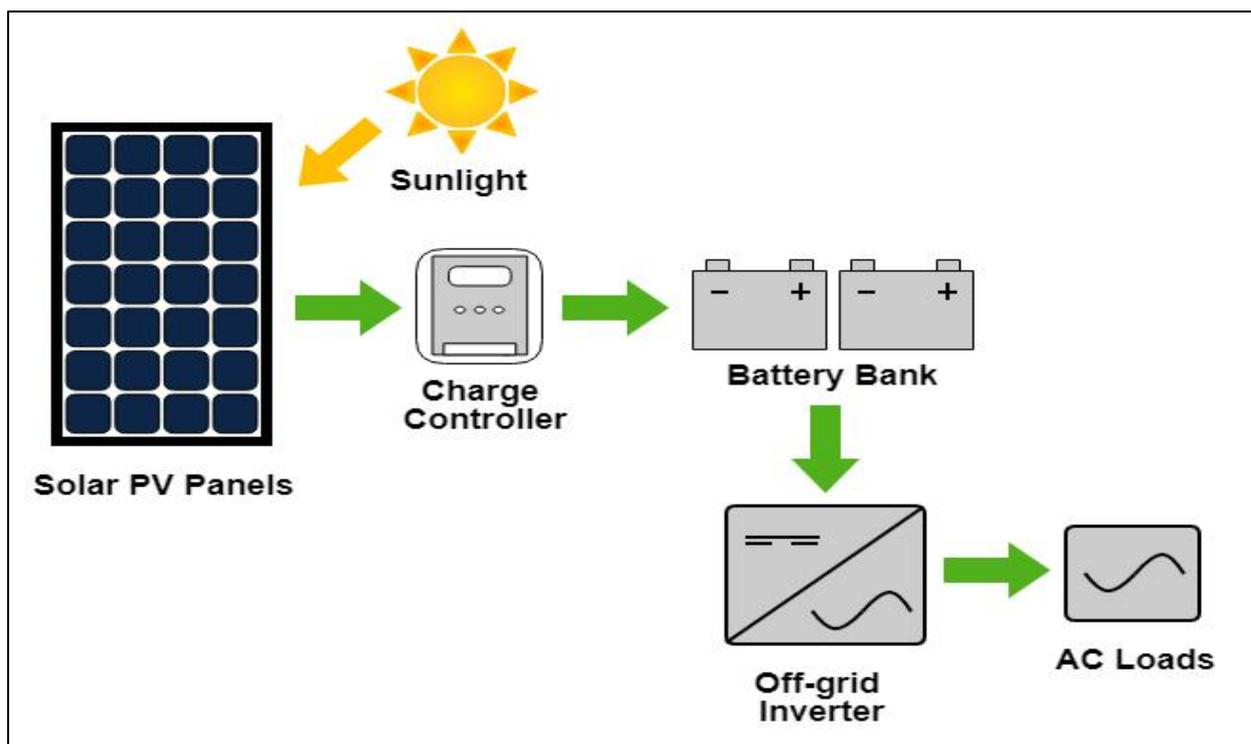
Figure 92: Stand-alone PV system (Source: Apricus solar)
