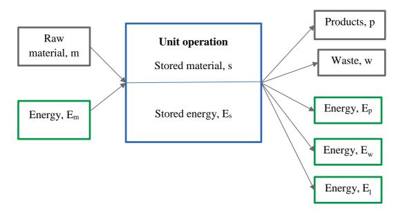
Figure 97: Energy and material balance representation
