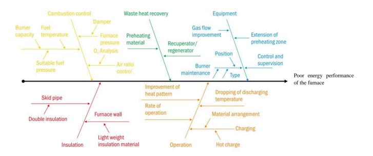
Figure 81: Fishbone diagram of fuel fired furnace for energy optimisation and control system improvement (Source: adapted from TERI)
