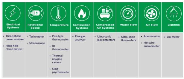
Figure 9: Appropriate portable measuring instruments for various systems
