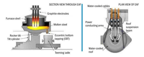
Figure 68: Electric arc furnace - section and plan view (source: steeluniversity.org)
