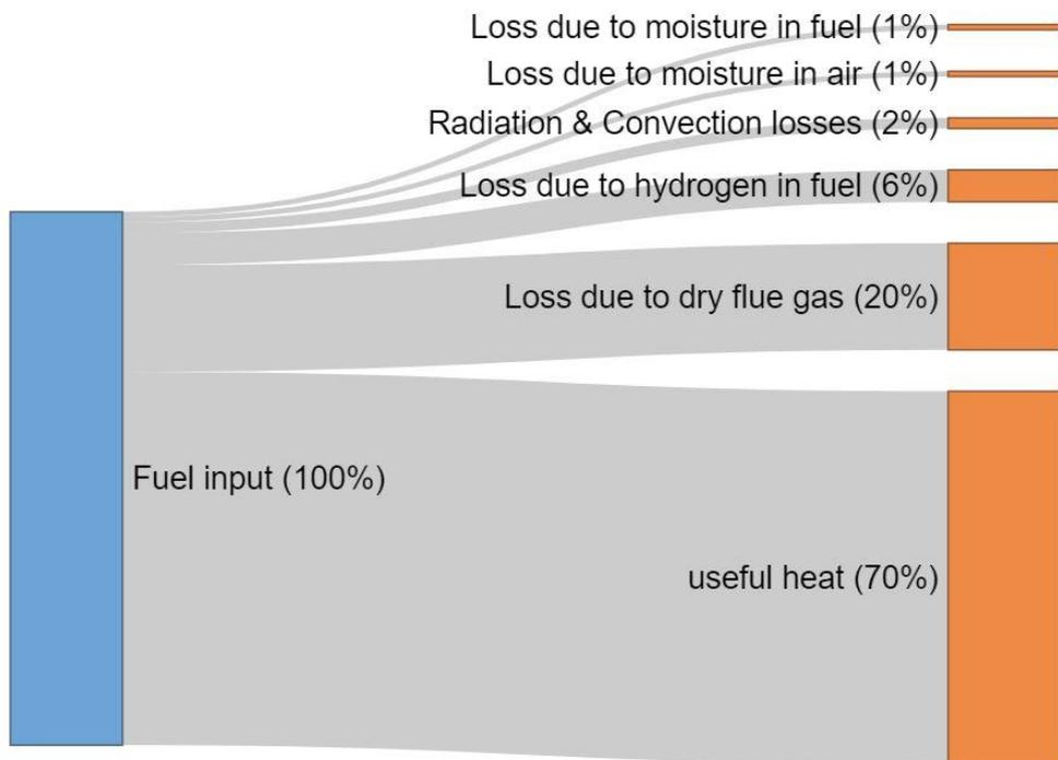
Figure 101: Sankey diagram for Boiler fuel input to heat output
