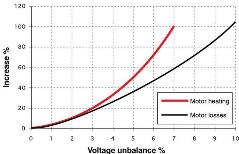
Figure 19: Voltage unbalance (%) versus motor losses & motor heating (Source: BEE)
