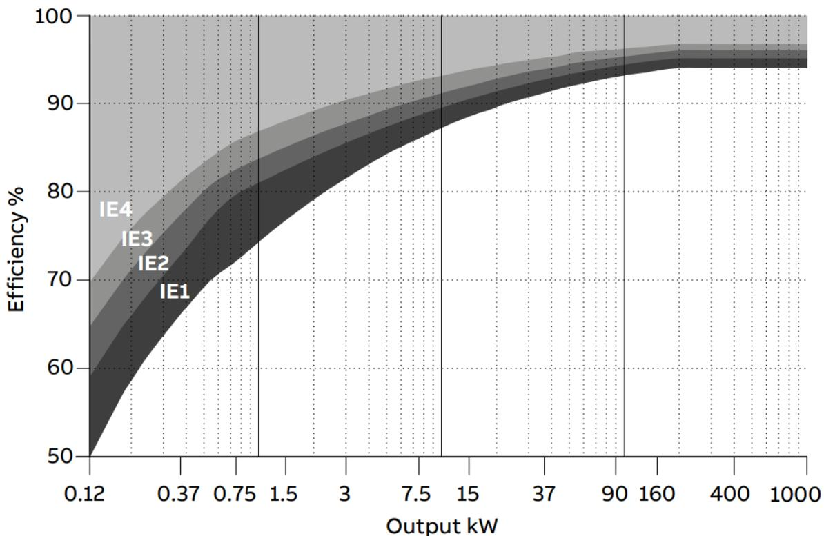
Figure 27: IE efficiency classes for 4 pole motors at 50 Hz (Source: ABB)
