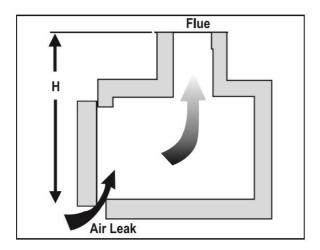
Figure 73: Air infiltration in furnace
