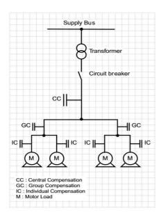
Figure 17: Different compensation modes for power factor improvement
