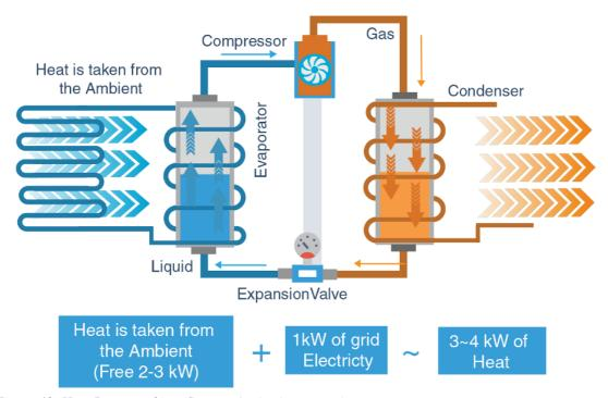
Figure 40: Heat Pump working (Source: Aspiration energy)
