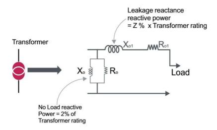
Figure 15: No-load compensation for transformer
