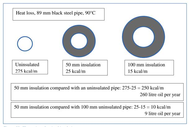
Figure 89: Illustration of optimal insulation
