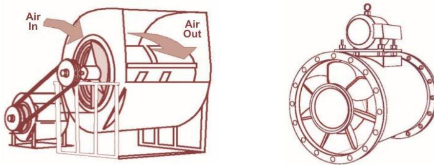
Figure 41: Centrifugal fan (left) and axial fan (right)
