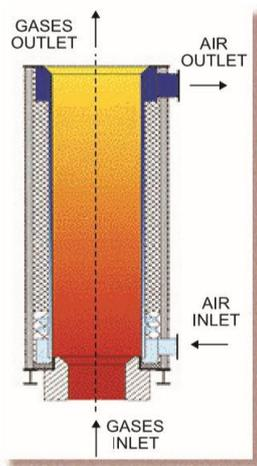
*Figure 84: Metallic radiation recuperator*
