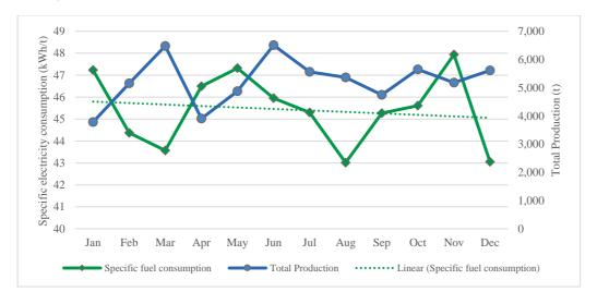
Figure 7: An example of line graph depicting specific fuel consumption (SFC) over time and decreasing trend of SFC
