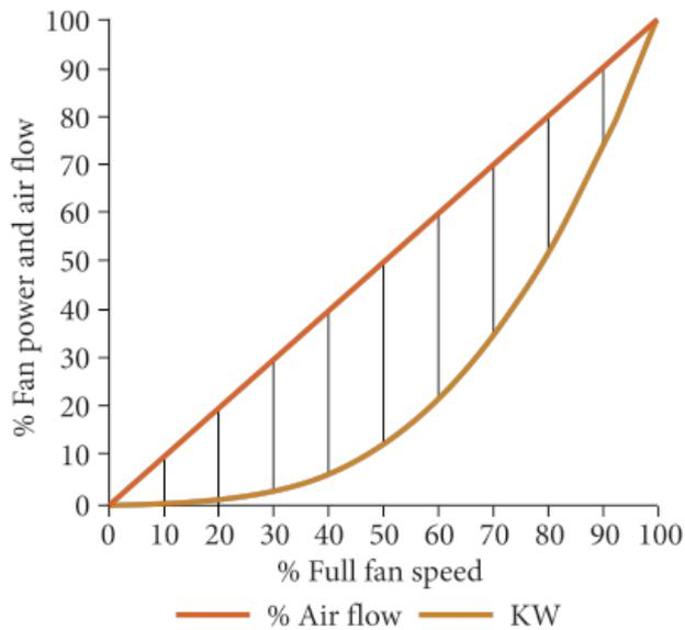
Figure 39: Effect of speed on power and air volume
