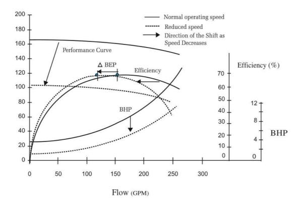
Figure 57: Effect of VFD
