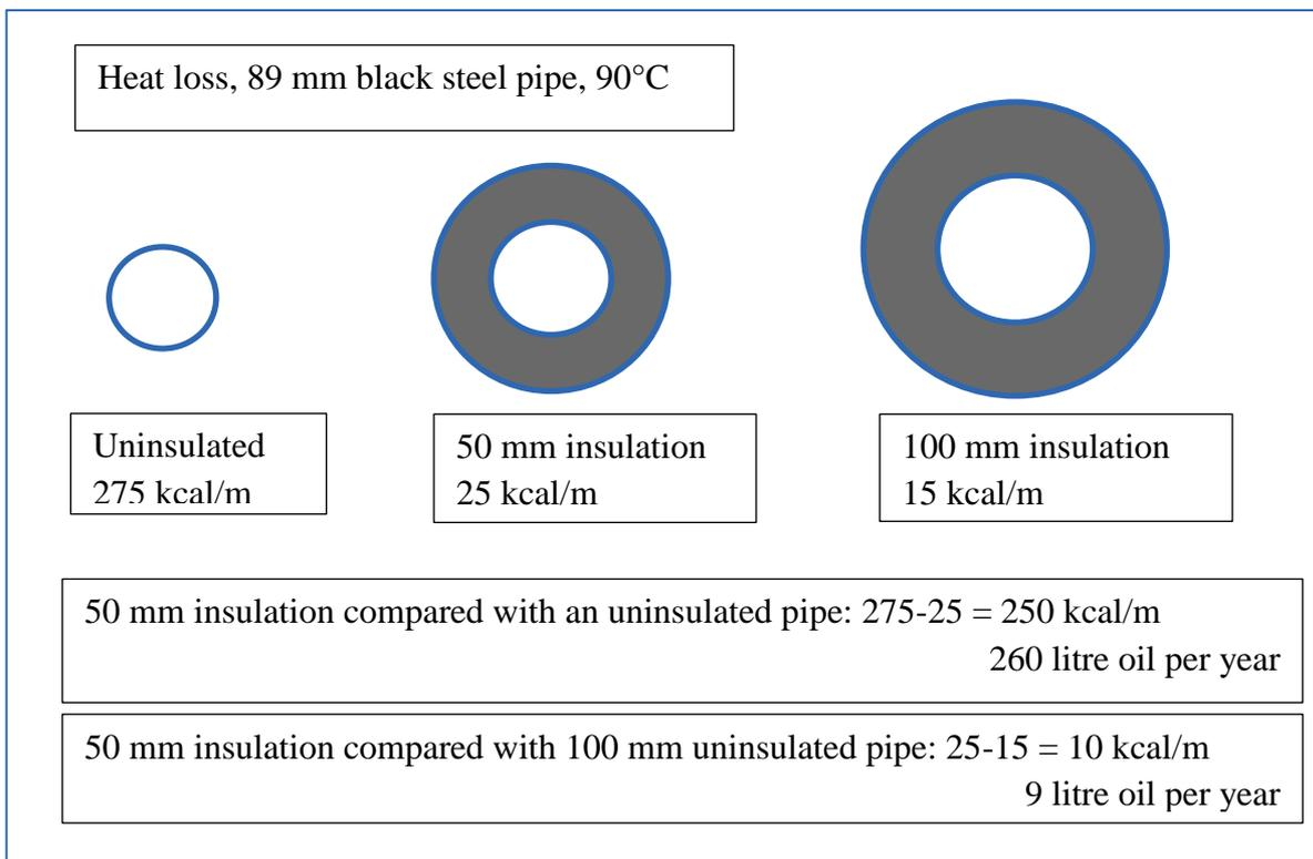
Figure 89: Illustration of optimal insulation
