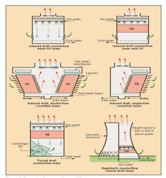
Figure 60: Types of cooling tower (Source: BEE)
