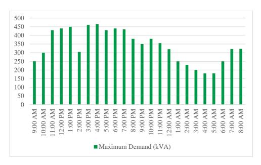
Figure 11: Hourly load curve
