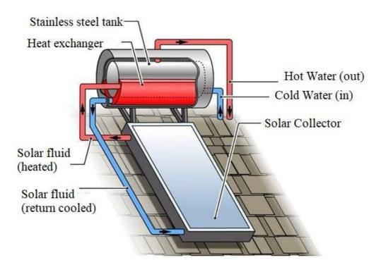
Figure 96: Solar water heater
