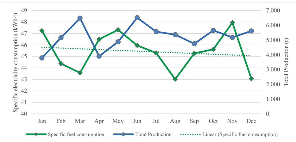
Figure 7: An example of line graph depicting specific fuel consumption (SFC) over time and decreasing trend of SFC
