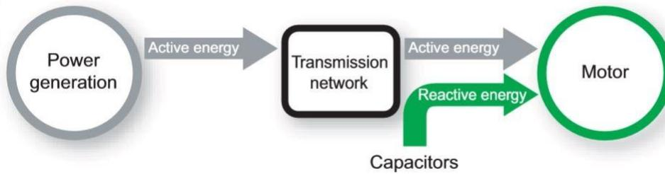
*Figure 14: Connection of capacitors at load level*
