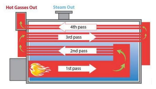
Figure 62: Fire tube boiler
