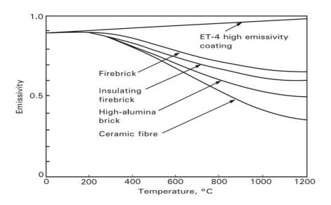
Figure 91: High emissivity coatings of various insulating materials
