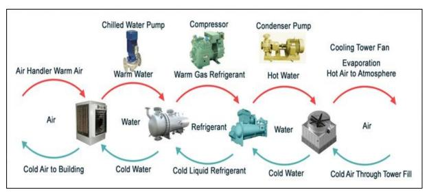
Figure 34: Heat Transfer Loops in refrigeration system
