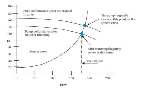
Figure 54: After impeller trimming
