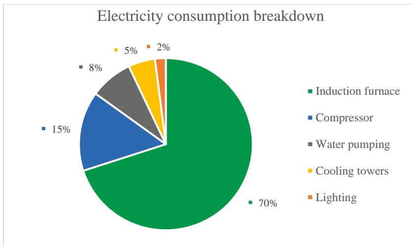
Figure 8: An example of electricity consumption breakdown
