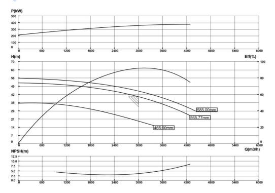
Figure 51: Typical pump curve provided by manufacturer
