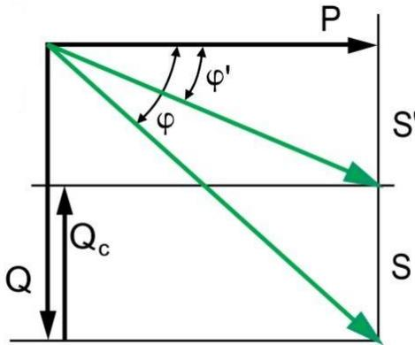
*Figure 16: Power factor correction triangle*
