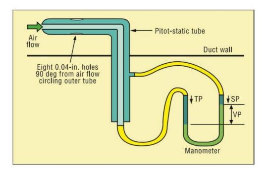
Figure 42: Measurement by pitot tube
