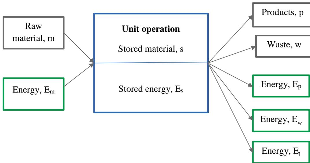
Figure 97: Energy and material balance representation
