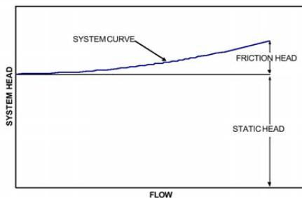
*Figure 48 System curve with high static head*
