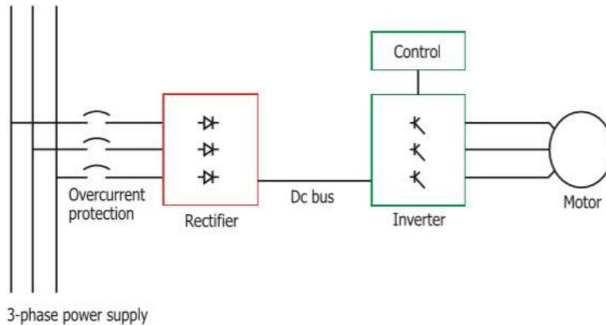
Figure 28: Component of VFD system
