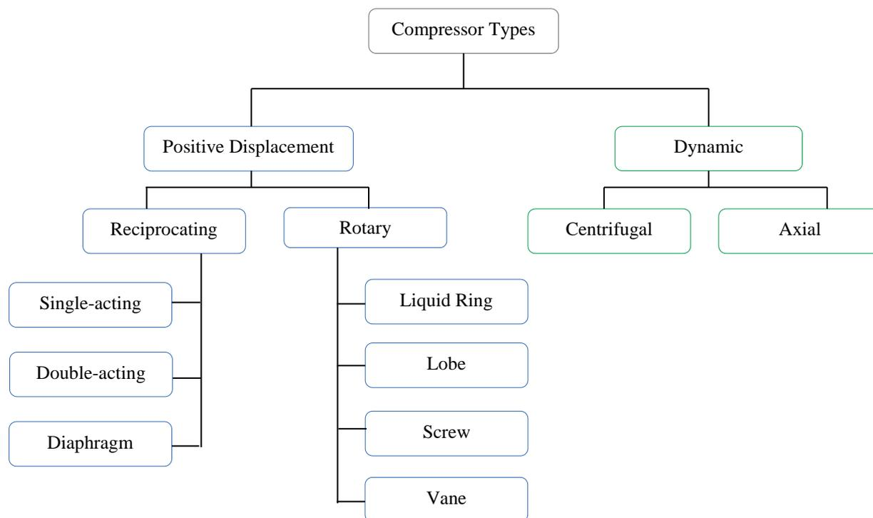
Figure 32: Types of compressors
