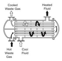
Figure 85: Tube type recuperator
