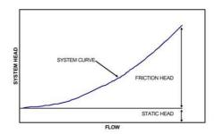
Figure 49 System head with low static head
