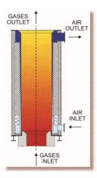
Figure 84: Metallic radiation recuperator
