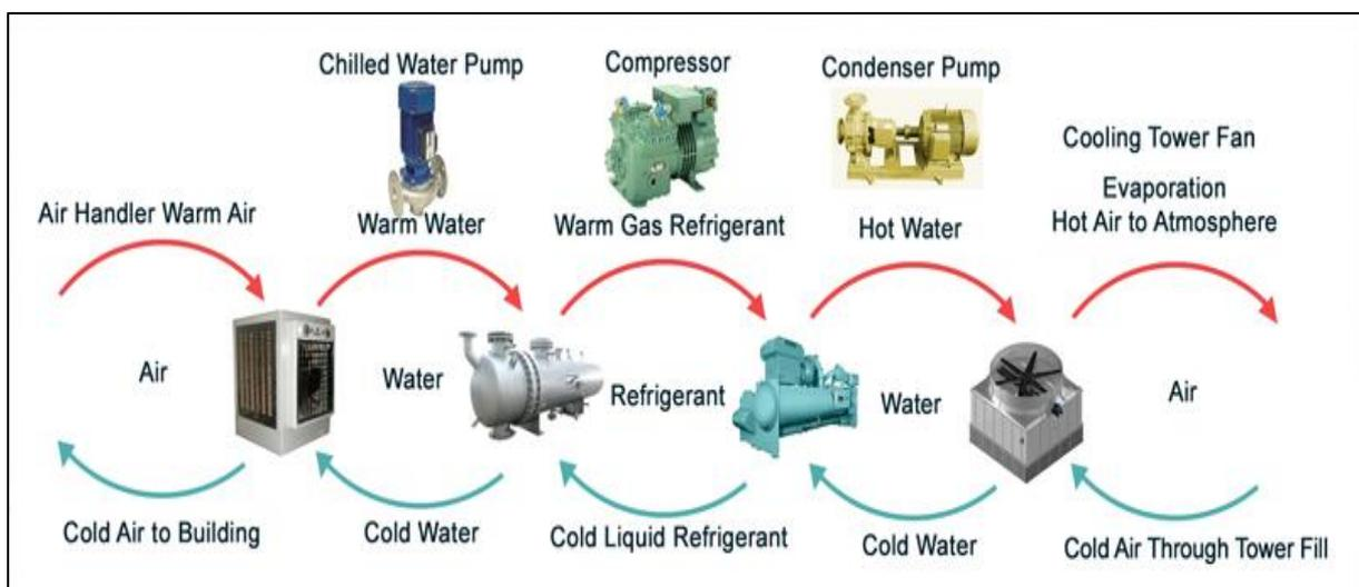
Figure 34: Heat Transfer Loops in refrigeration system
