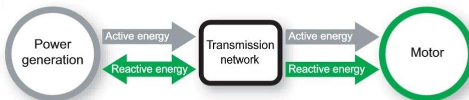
Figure 12: Reactive energy supplied and billed by the energy supplier or utility
