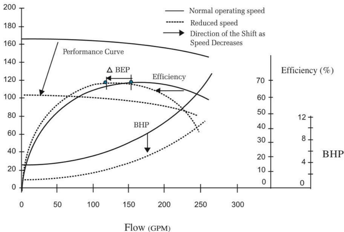
Figure 57: Effect of VFD
