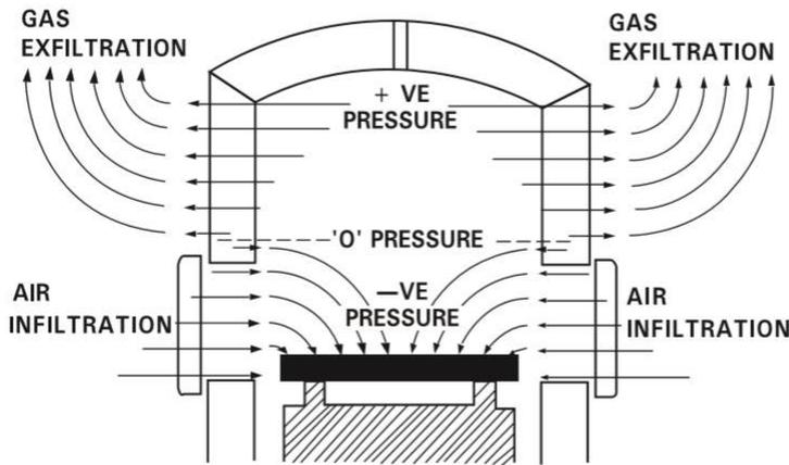
Figure 78: Effect of pressure on the location of zero level and infiltration of air (Source: BEE)
