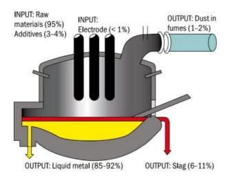
Figure 69: Material balance of EAF
