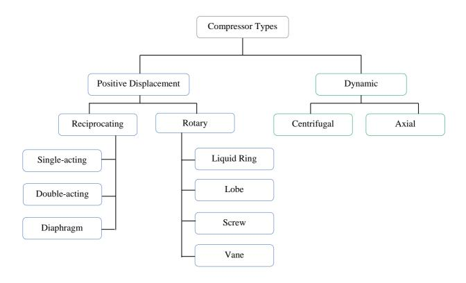
Figure 32: Types of compressors
