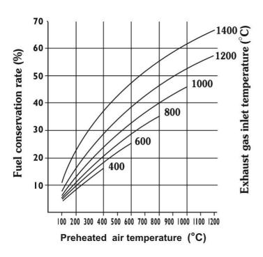
Figure 80: Fuel savings rate by preheated air temperature (Source: BEE)
