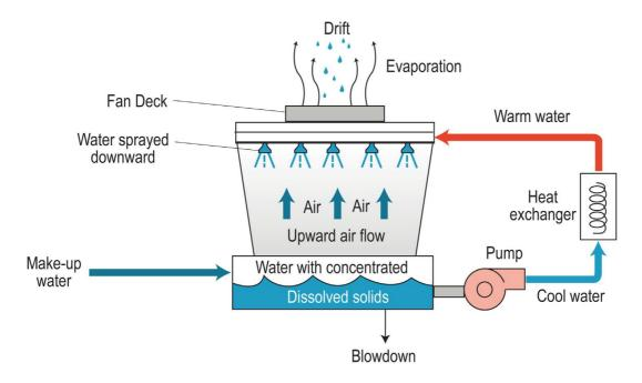
Figure 59: Cooling tower with closed loop
