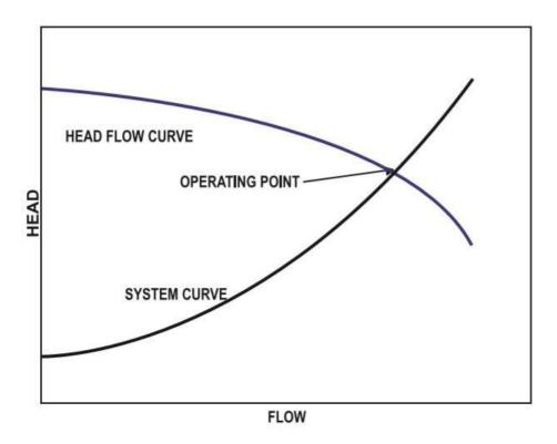
Figure 52: Pump operating point
