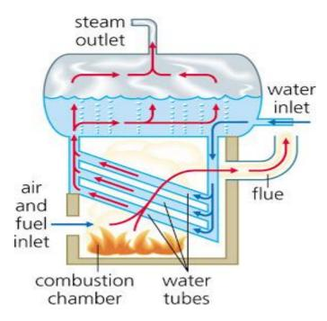
Figure 63: Water tube boiler (Source: BEE)
