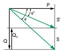
Figure 16: Power factor correction triangle
