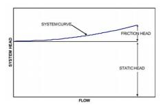
Figure 48 System curve with high static head
