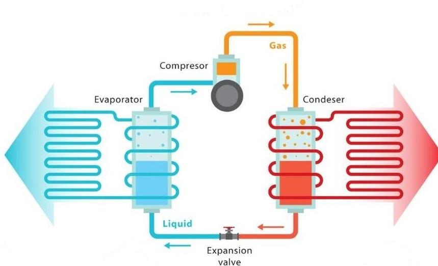
Figure 37: Vapour compression refrigeration system
