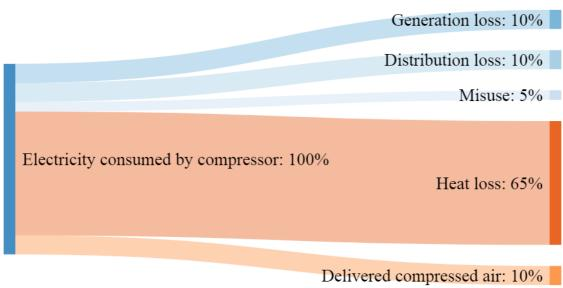
Figure 31: Sankey diagram of compressed air losses
