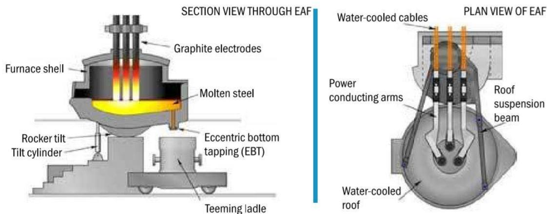
Figure 68: Electric arc furnace - section and plan view (source: [steeluniversity.org](http://steeluniversity.org))
