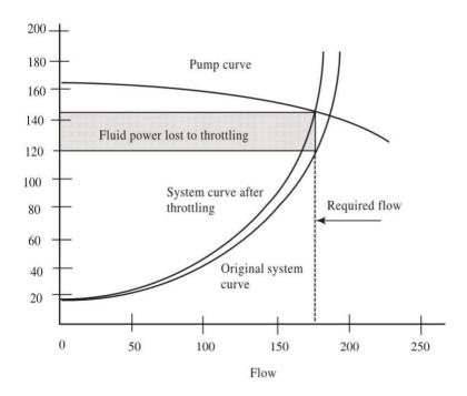
Figure 53: Before impeller trimming
