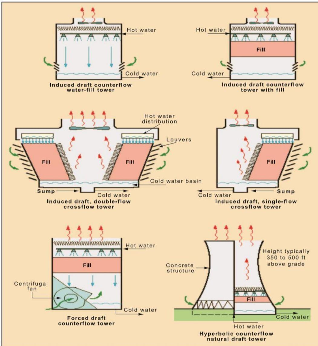
Figure 60: Types of cooling tower (Source: BEE)
