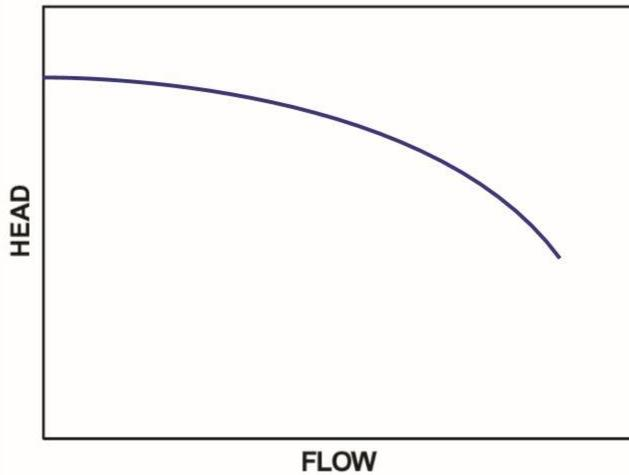
Figure 50: Head-Flow curve
