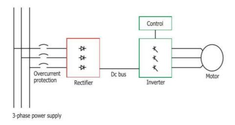
Figure 28: Component of VFD system
