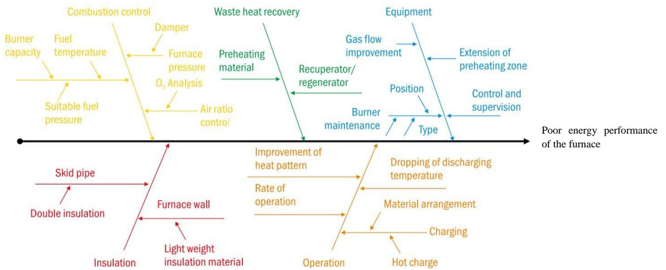
Figure 81: Fishbone diagram of fuel fired furnace for energy optimisation and control system improvement (Source: adapted from TERI)
