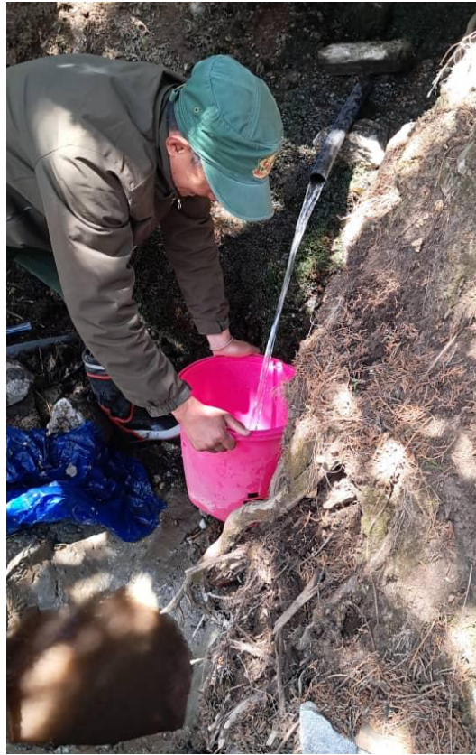
Figure 156: Volumetric/Bucket method (Photo-Kinley Dem, DoW)
